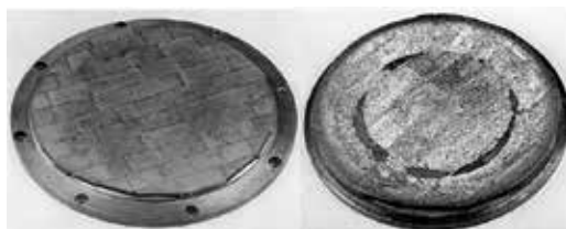
Figure 18. Composite WSi 2 targets for magnetron sputtering: left, new; right, after 150 cycles.
