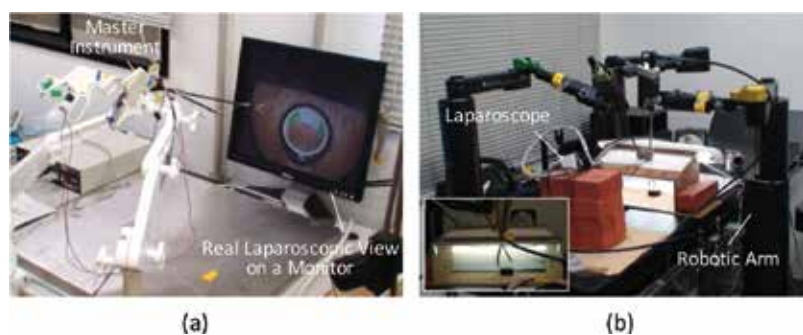
Figure 5. Object-touching task during the task in iSPS: (a) master set-up and (b) slave set-up.
