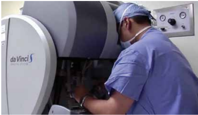
Figure 1. Surgeon operating at the ergonomic console unit (“master interface”). The user interface allows for “endowrist” articulation of instruments, with seven degrees of freedom for motion.
