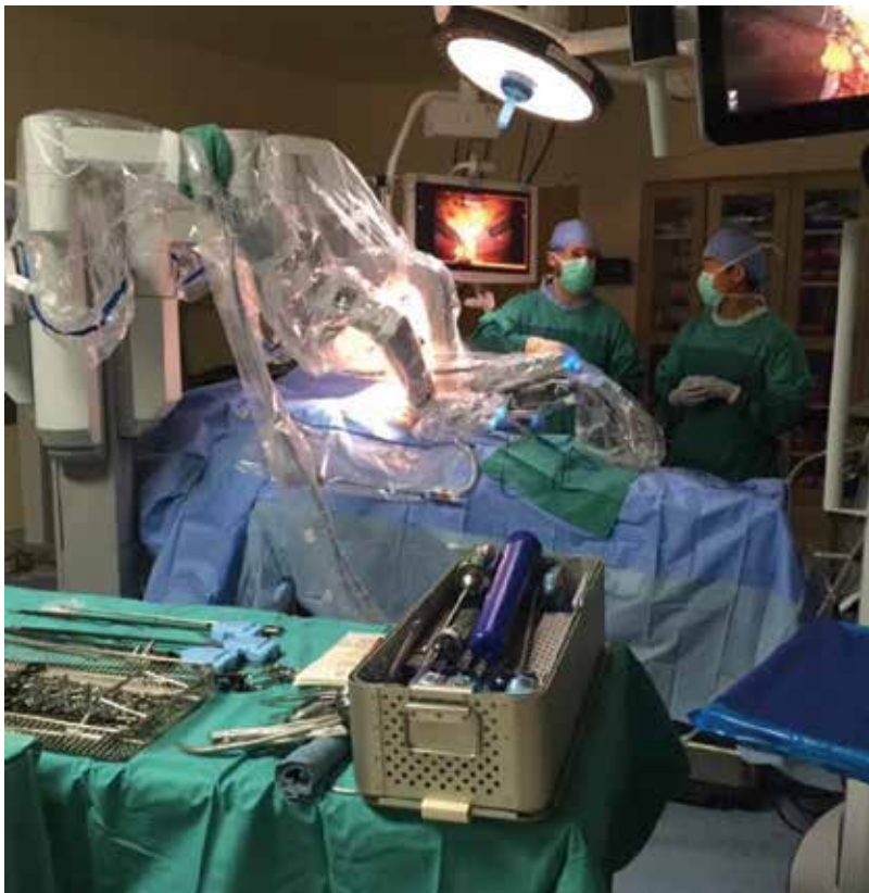
Figure 2. da Vinci system (“slave manipulator”) with robotic arms already docked and executing the tasks with the surgeon in control, with the surgical team at the bedside.
