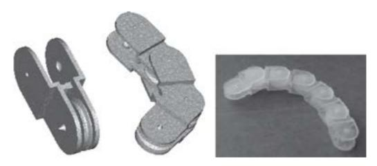
Figure 21. Snake-like mechanism with built-in joints and pulleys. CAD model of a single segment (left) and of two connected segments (center) and prototype (right)
