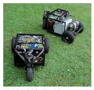
Figure 10. Completed mobile platforms, "itchy" and "scratchy"
