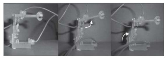
Figure 23. 2R Robot Actuated
