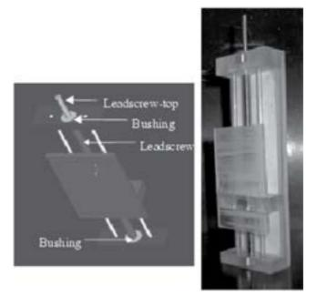
Figure 25. Elevator Model with 4 Embedded Components
