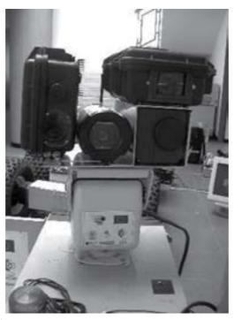
Figure 9. Detail of the pan-tilt turret
