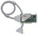
Figure 7(b). A DAQ card with cable
