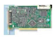
Figure 7 (a). A DAQ PCI card Figure 7. Multifunction NI DAQ PCI 6024E card with application
