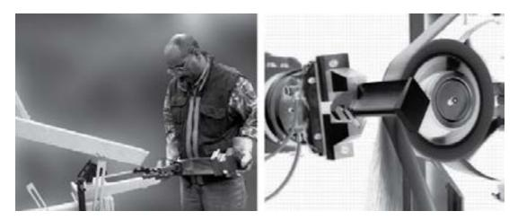
Figure 2. Manual grinding process and robot aided grinding process
