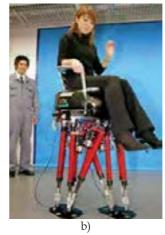
Figure 8. Waseda biped locomotor WL-16R with non anthropomorphic legs: a) a side view; b) carrying a human
