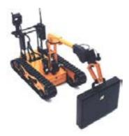
Figure 2. RoboProbe Technologies Inc. bomb disposal robot
