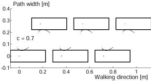
Figure 26. Mechanism footprints of decelerated motion for c = 0.7. No compensation applied.
