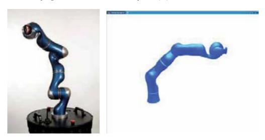
Figure 1. DLR-Lightweight-Robot-III. The picture on the right hand side shows the initial configuration of the robot in the simulation study
