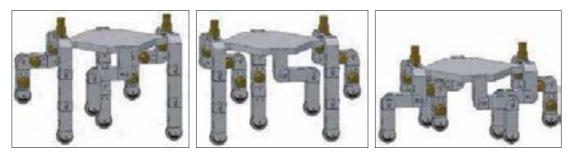
Figure 28. An application of the proposed low-cost modular anthropomorphic leg for hexapod walking machines
