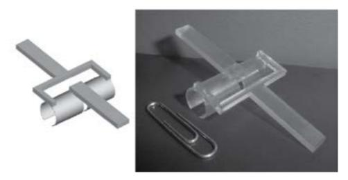
Figure 20. Virtual and Fabricated Compound Split Tube Model
