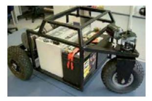
Figure 9. Complete chassis and drive components
