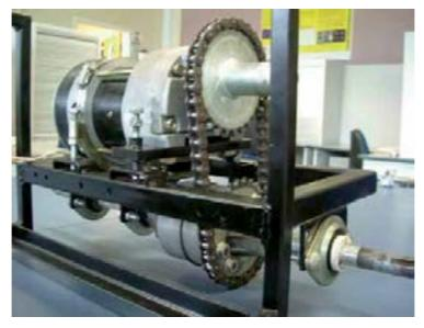
Figure 7. Mounted drive system showing chain tensioning method
