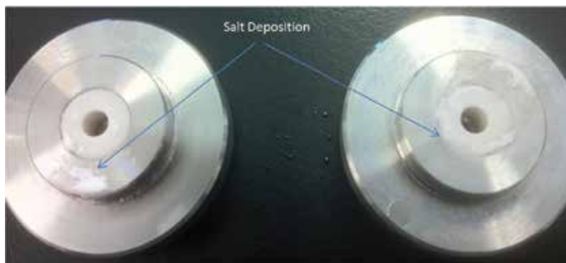
Figure 36. Salt depositions at screws of the column.
