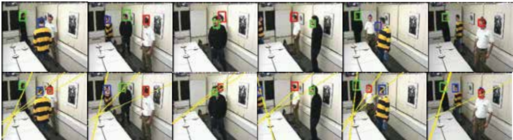
Figure 6. AV16.3, sequence 45 camera #3: occlusions with three speakers [14]. The tracking results of the V-SMC-PHD and the AV-SMC-PHD filters are shown in the first and second rows, respectively.
