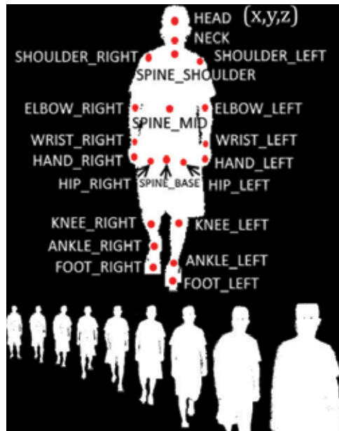
Figure 8. Two kinds of data in our database: 3D position of 21 joints in the upper area and the corresponding binarized silhouette images in the lower area.
