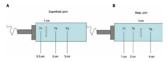
Figure 1. Scheme of the phantoms mimicking a superficial (A) and a deep (B) joint indicating the position of the bone insert and of the temperature probes.
