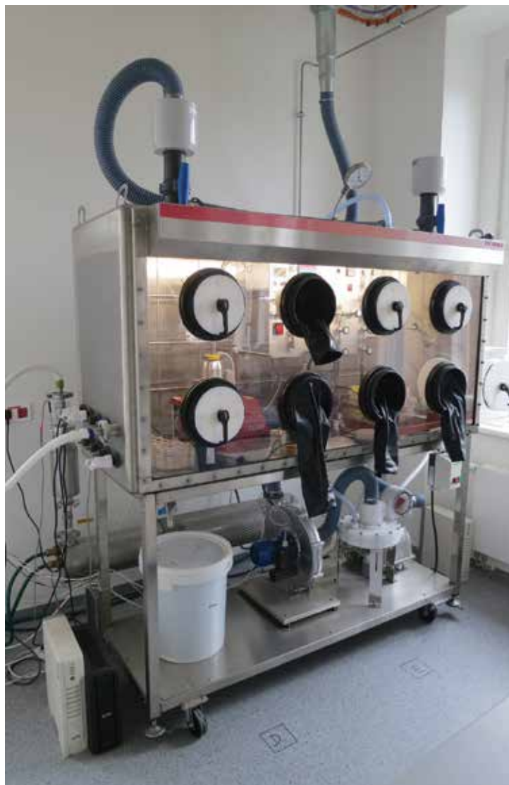
Figure 15. The equipment for safe handling of tritium gas; the tritium manifold (RC-TRITEC AG) placed in the glove box; a scrubber for decontamination placed behind the glove box.
