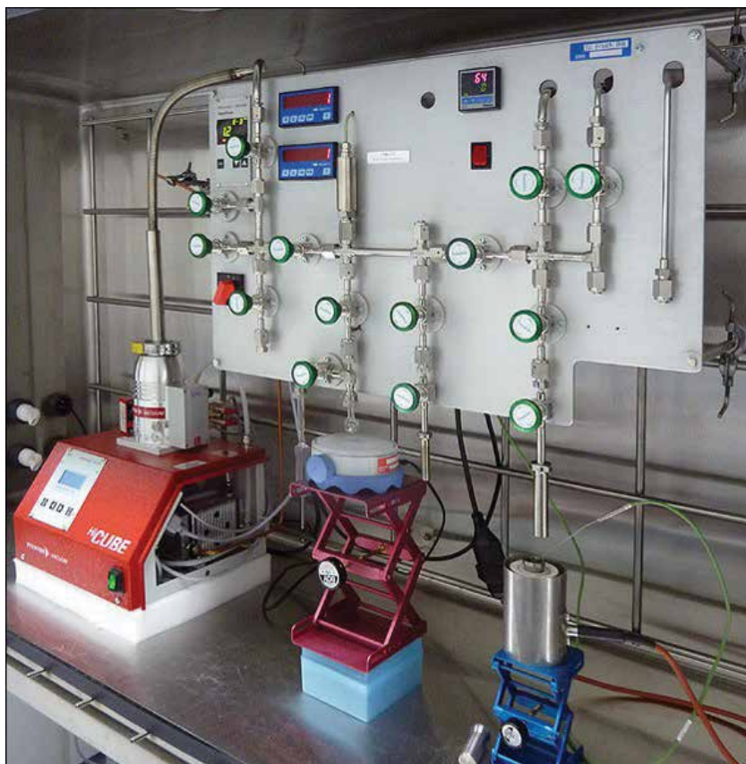
Figure 16. The equipment for safe handling of tritium gas; the tritium manifold (RC-TRITEC AG) placed in the glove box.
