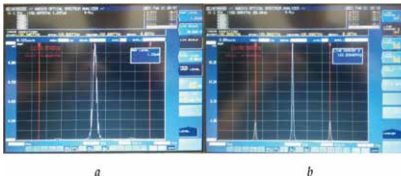
Figure 12. The spectrogram of the signal in destructive (a) and constructive (b) interference on the lateral frequencies \omega \pm \Omega in PM-PM scheme implementation.
