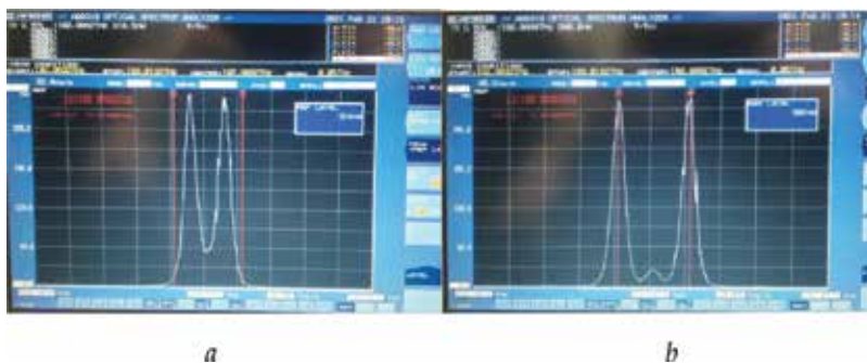
Figure 14. The output spectrum of AMPC procedure for propagation in FOLC: frequency encoding of second | -; 1\rangle and third |+; 2\rangle photon states is shown.
