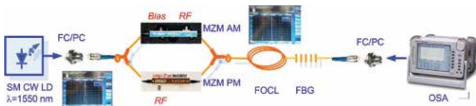
Figure 7. Schematic representation of a general parallel single-port filtered MWP link [25].
