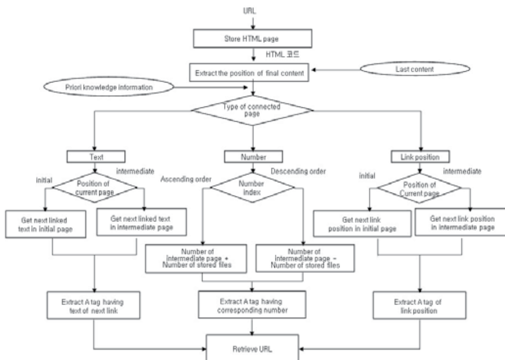
Fig. 5. Extracting URL Flow for the connected web documents.
