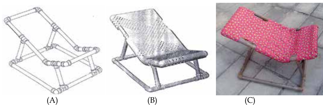
Fig. 10. (A) and (B): PVC pipes and connections structure; (C) Final craft model.
