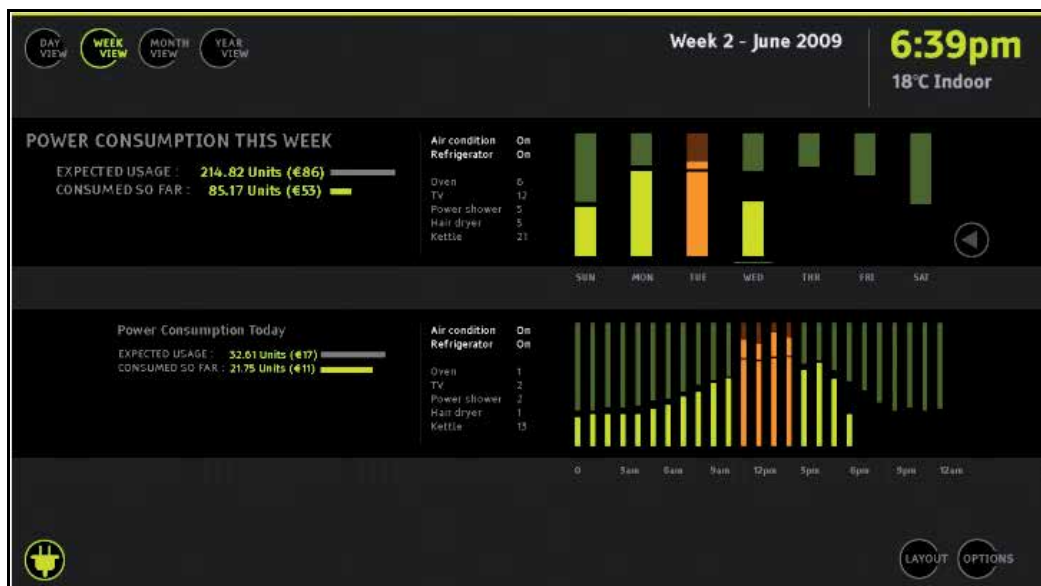
Fig. 5. Example of dark background with bright information; In-home display electricity monitor, Doherty et al. (2010).
