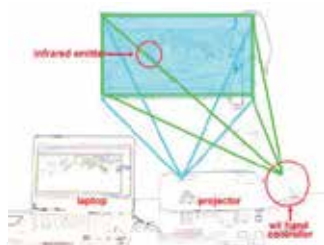
Fig. 1. How to use the low-cost interactive whiteboard on a wall
