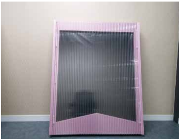
Figure 9. One square metre effective area MES prototype with 10 layers, whose weight is 15 kg.
