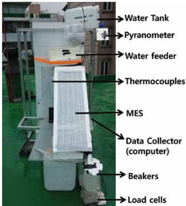
Figure 12. Experimental setup of the prototype MES outdoor test.
