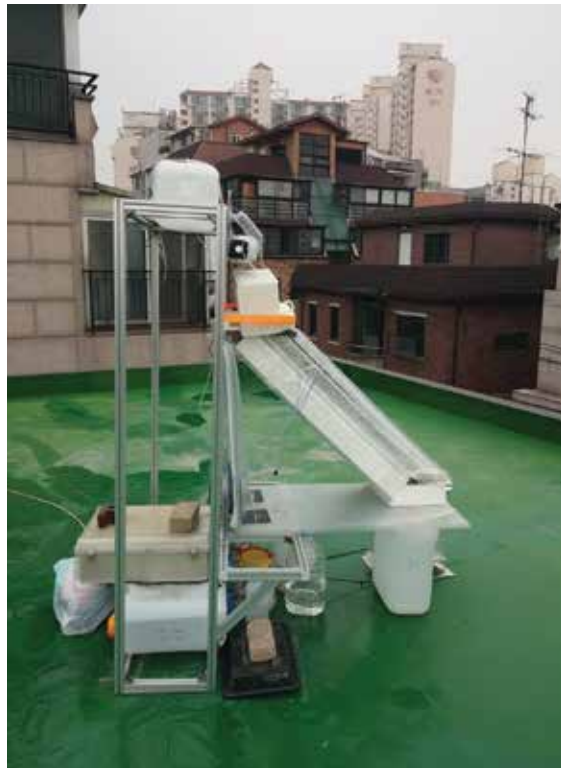
Figure 8. MES system installed tilted 45°.
