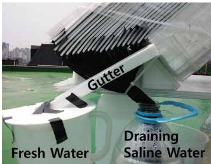
Figure 11. Collecting fresh water from each layer by a gutter.
