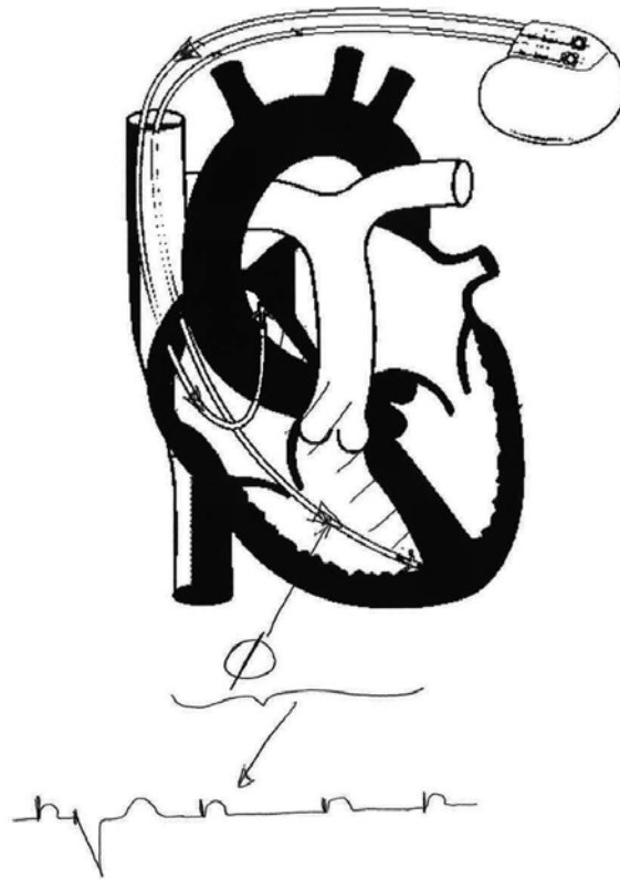
Figure 16. Crosstalk: atrial activation is sensed on the ventricular channel resulting in inhibition of ventricular pacing.
