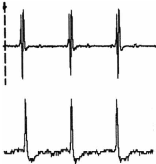
Figure 7. Raw and filtered electrograms sensed by a pacemaker. The top tracing is the filtered signal used by the pacemaker for sensing. Filtering of the raw signal is necessary to prevent (over)sensing of the T-wave, far-field signals, and myopotentials.
