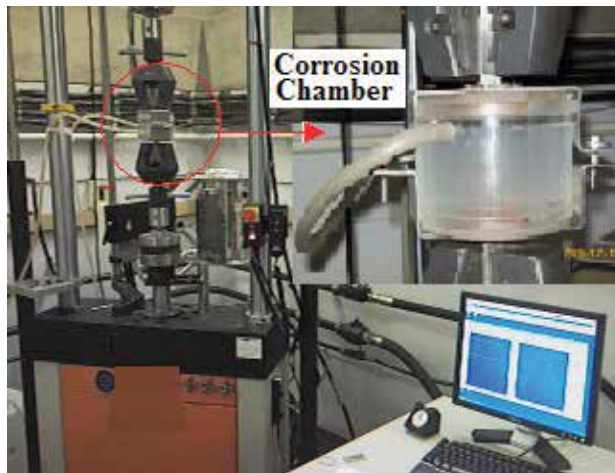
Fig. 10. The experimental set-up used for corrosion fatigue testing in a NaCl solution.
