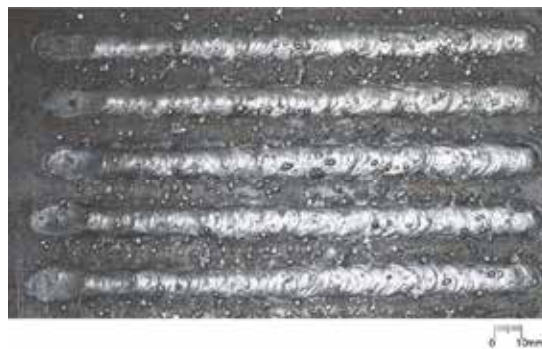
Fig. 10. Beads on plate performed by the robot using E6013 electrodes, demonstrating the repeatability of the process.
