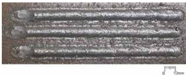
Fig. 11. Welds made using E7018 electrodes demonstrating the flexibility and repeatability of the process.
