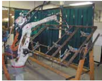
Fig. 17. Tests at University laboratory for verification of the welding parameters.
