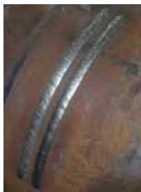
Fig. 13. Welds made on tube with E7018 electrodes.
