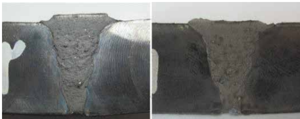
Fig. 7. Front view of the weld sections, 32.3\text{J}/\text{mm}^2 WHI and 393\text{ J}/\text{mm} heat input according to Ex. 1 parameters (left); 35.2\text{J}/\text{mm}^2 WHI and 337\text{ J}/\text{mm} heat input with Ex. 2 parameters (right)
