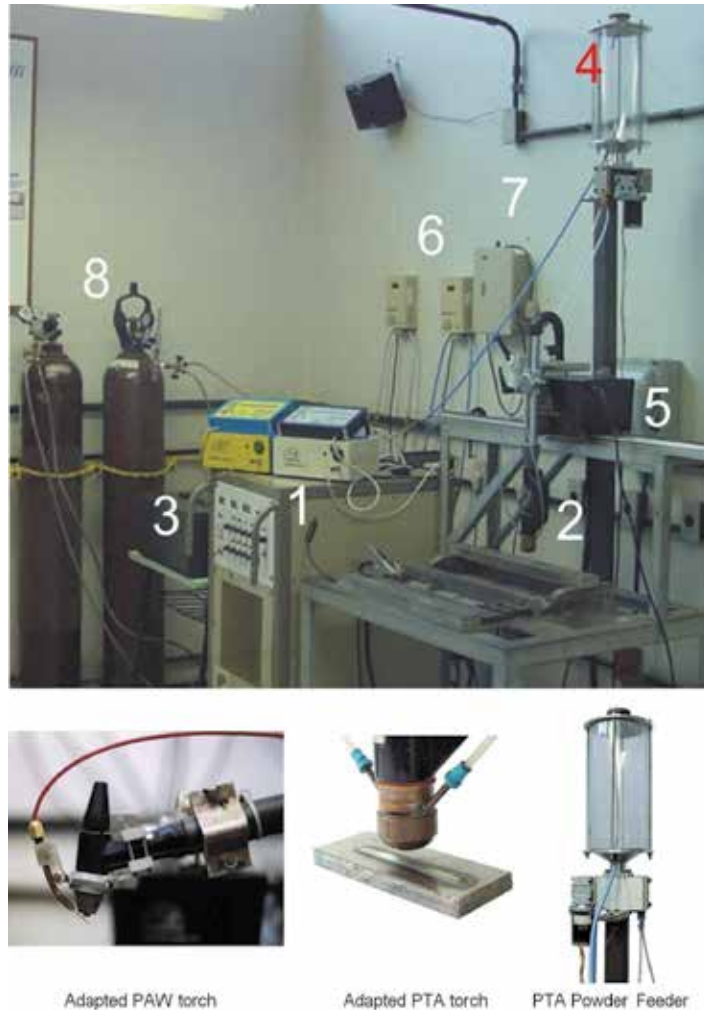
Fig. 3. Test bench assembled at the welding laboratory. 1-Welding source; 2-Adapted plasma torch; 3-Plasma module; 4-Powder feeder; 5-Torch displacement system; 6-Digital gas meters; 7-Electronic gas valve; 8-Gases
