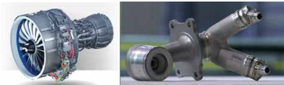
Figure 12. The LEAP engine (to left) has 19 3D-printed fuel nozzles (top right) and static turbine shrouds made from ceramic matrix composites (CMCs) (above left). Image credit: CFM.
