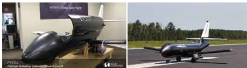
Figure 14. 3D-printed military drone-PTERA of solid concepts.
