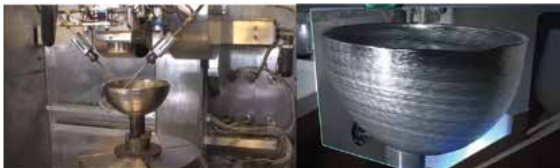
Figure 13. The manufacturing procedure of one half of a satellite fuel tank according to the Sciaky method (top left) and finished half-product (top right). Source: Sciaky Inc. Video capture.
