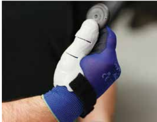
Figure 7. BMW has turned to 3D printing to augment its workers and stop strain on limbs frequently found on manufacturing lines. Photograph: BMW (republished from the Guardian).
