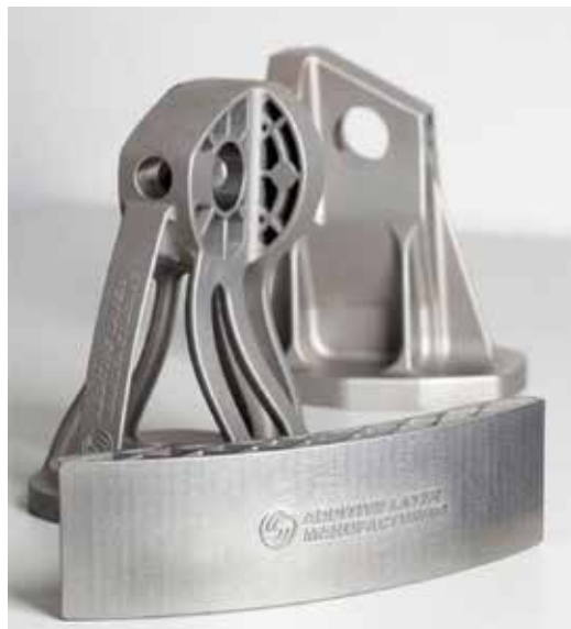
Figure 6. A stainless-steel bracket optimized for weight reduction (front) and the traditional cast bracket in the back. Source: European Space Agency events via Flickr.
