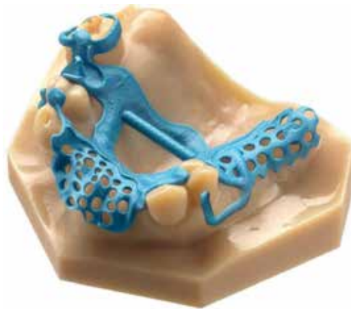
Figure 8. An example of a dental frame built using wax deposition modeling. Source: www.Stratasys.com.
