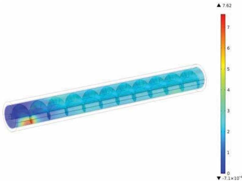
Figure 10. The calculated fields of steam concentrations.
