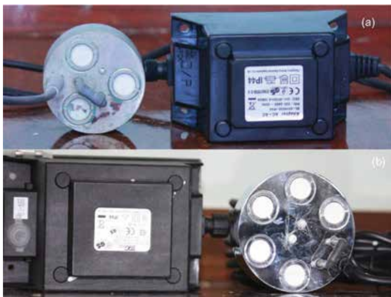
Figure 7. Ultrasonic nebulizers employed in the study: (a) shows the 1.7 MHz ultrasonic nebulizer with power supply unit and (b) shows the 4.8 MHz ultrasonic nebulizer with power supply unit.
