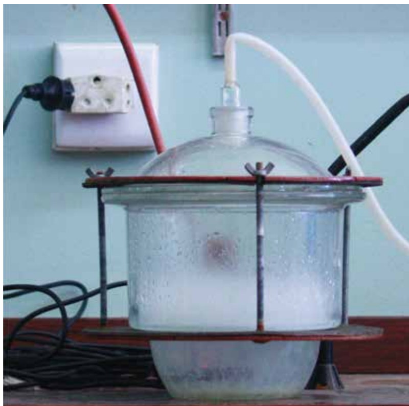
Figure 6. An actual photograph of the USP reaction vessel used.
