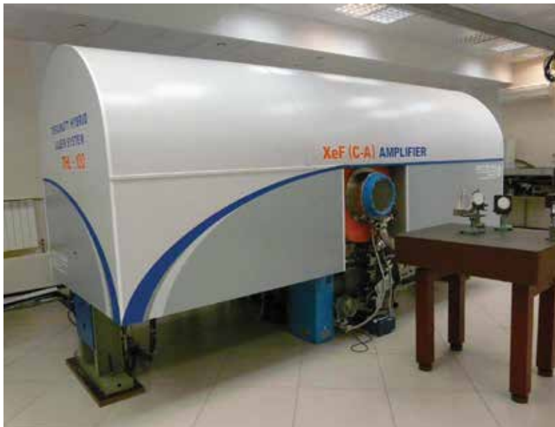
Figure 12. Photo of the XeF(C-A) amplifier.
