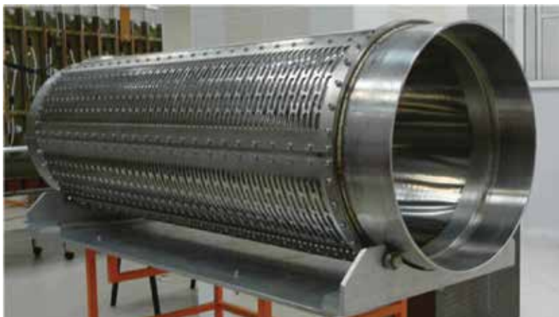
Figure 14. Gas chamber of the XeF(C-A) amplifier with windows for electron beam injection.
