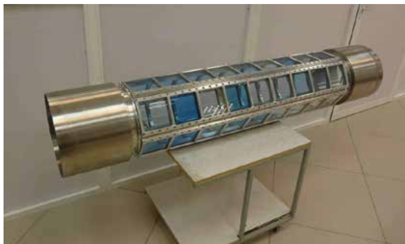
Figure 15. Laser cell of the XeF(C-A) amplifier.
