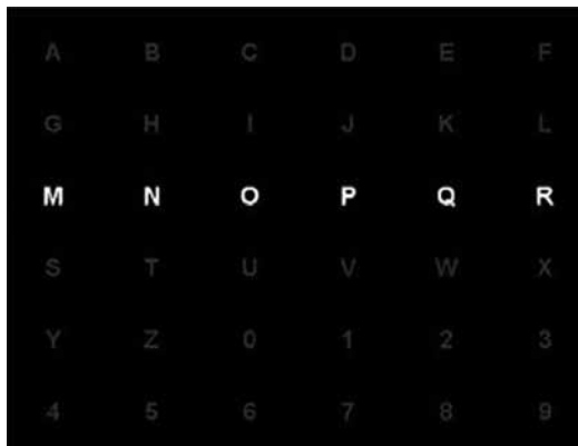
Figure 3. The row-column (RC) paradigm. One row (MNO PQR) is flashing.
