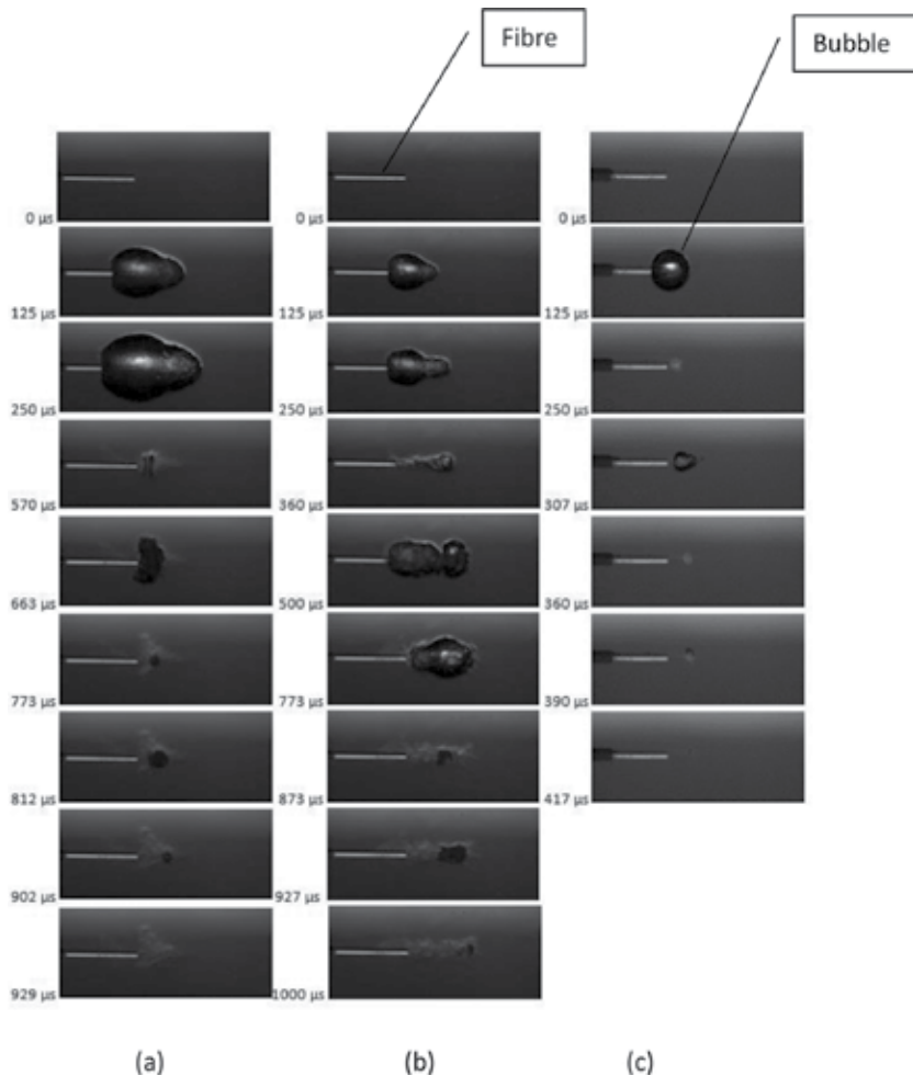
Figure 12. Series of screen shots of cavitation bubbles behavior of Ho and Tm lasers. (a) Ho at 1 J and 150 \mu\text{s} ; (b) Ho at 1 J and 800 \mu\text{s} ; (c) Tm 0.02 J and 450 ns.
