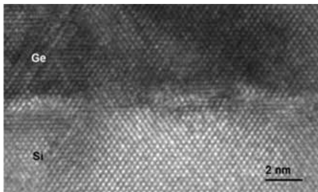
Figure 5. Atomic-resolution cross-sectional TEM image of Ge/Si interface on the sample deposited at 300°C.
