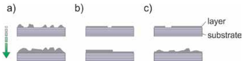
Figure 1. Modes of growth: (a) Volmer-Weber; (b) Frank-van der Merwe; and (c) Stranski-Krastanov.
