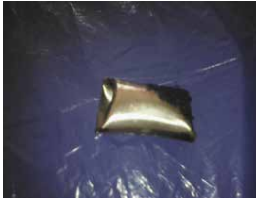
Figure 2. The mobile phone battery modified by the heat.
