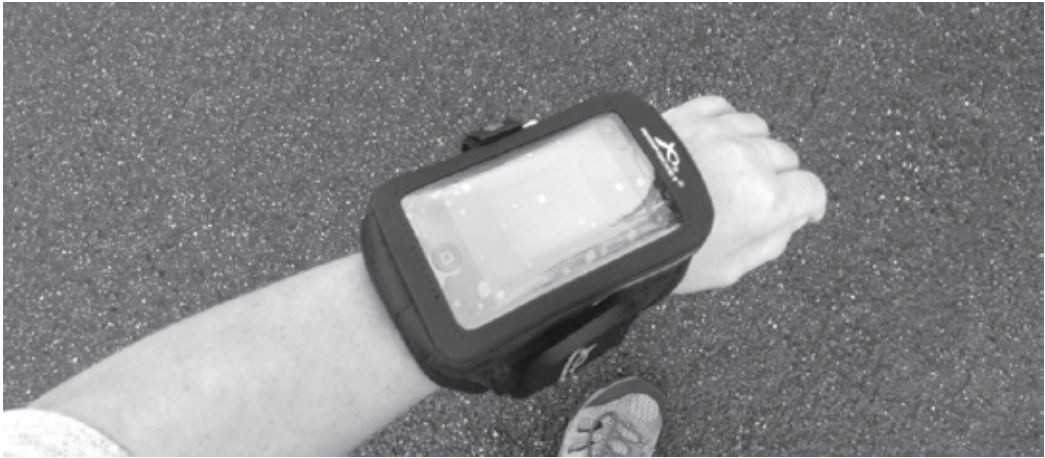
Figure 4. Mounting of the smartphone as a wireless gyroscope platform for quantifying reduced arm swing [49].
