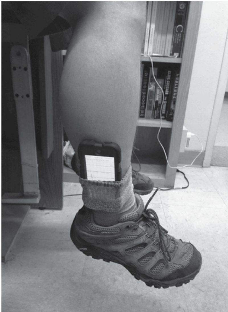
Figure 1. Portable media device as a wireless gyroscope platform for quantifying the patellar tendon reflex response [45].
