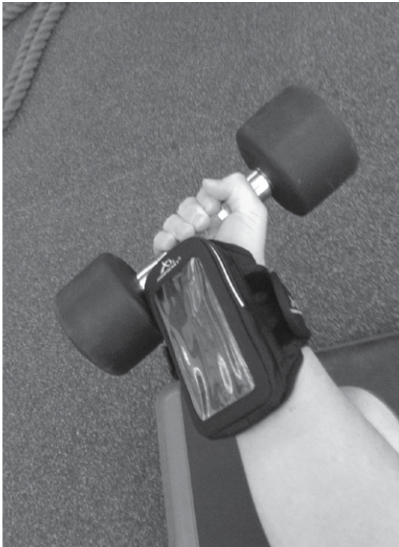
Figure 9. Virtual Proprioception for eccentric training demonstrated with a smartphone functioning as a wireless gyroscope platform secured proximal to the wrist through an armband [54].
