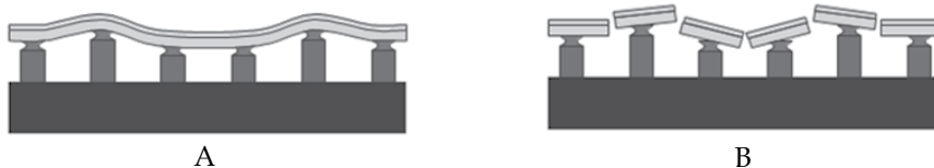
Fig. 7. Deformable mirror (DM) types. (A) Continuous surface mirror, deformed by an underlying array of actuators. (B) Segmented surface - the mirror is composed of a discrete array of segments each of which has three degrees of freedom: piston, tip and tilt (PTT). Piston only segmented DMs are also possible.
