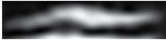
Fig. 9. Low-frequency illumination distribution of a typical bright and dark moiré fringes.
