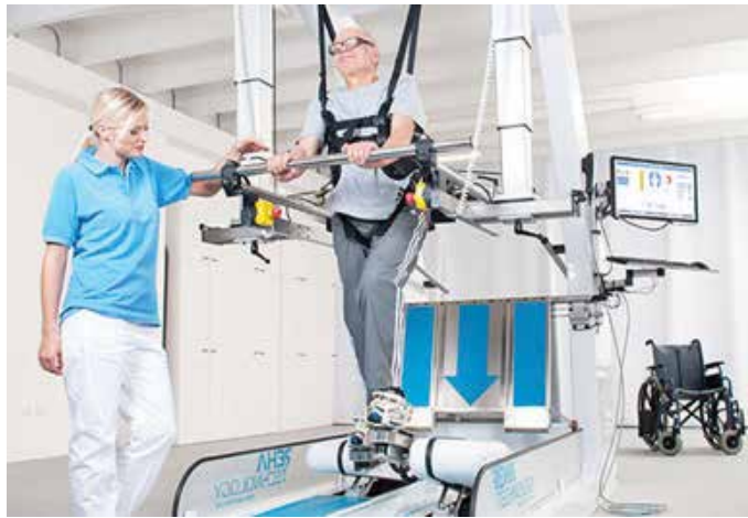
Figure 11. The G-EO system for gait rehabilitation.
