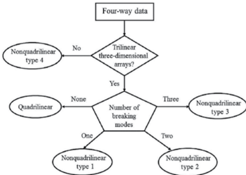
Figure 3. Classification tree for four-way data for a set of samples, according to whether the individual three dimensional arrays data are trilinear or not and to the number of quadrilinearity-breaking modes [26].
