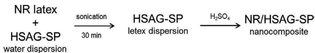
Scheme 4. Procedure for the preparation of NR/HSAG-SP nanocomposite from NR latex.
