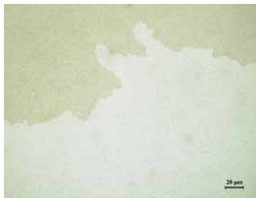
Figure 6. Example of a structure surface with Co layer 300 nm thick annealed at 990°C for 60 s. (Reprinted with permission from J Mater Sci: Mater Electron, No. 3995250684677.).
