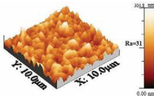
Figure 3. AFM picture of the graphene film surface prepared on the Ni(300)/SiC structure annealed at 1000°C for 120 s. (Reprinted with permission from J Electrical Engineering.)
