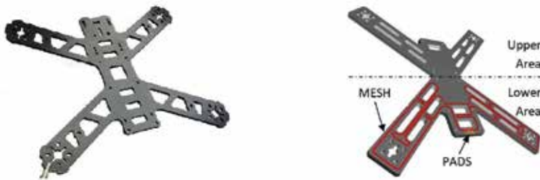
Figure 4. Traditional drone frame (left), enhanced NDT CAD frame (right).
