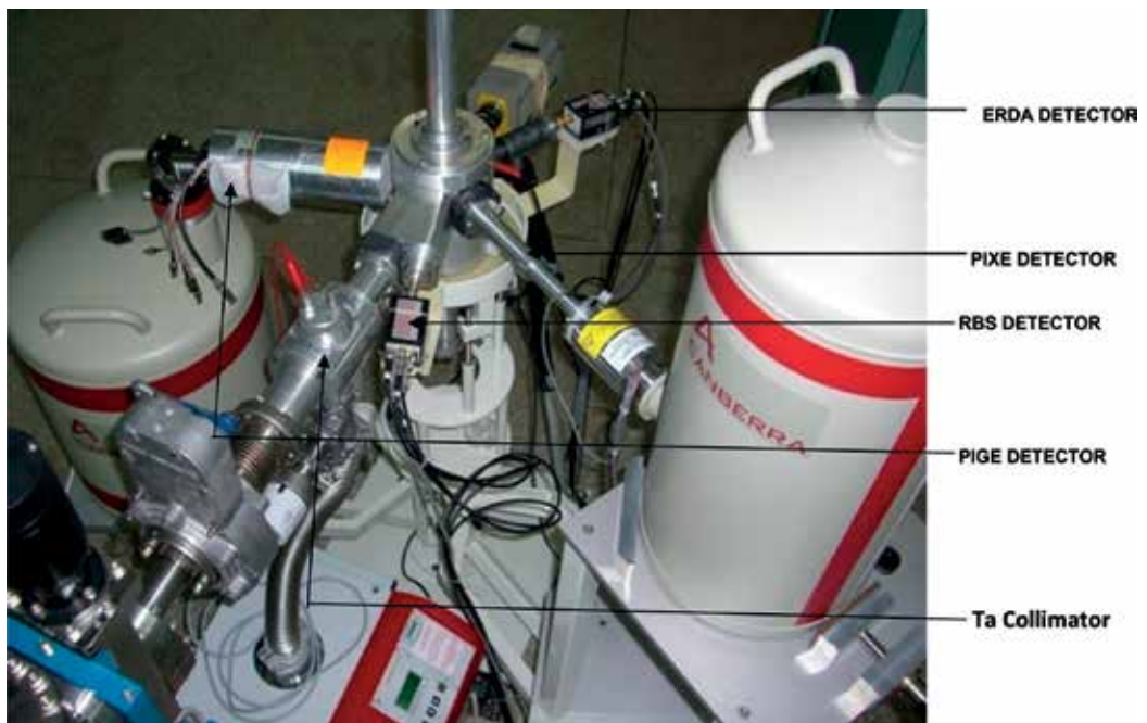
Figure 3. General view of the IBA End Station at CERD, OAU, Ife, Nigeria showing four ports and a window for RBS, PIXE, ERDA, and PIGE detectors (Source: [13]).
