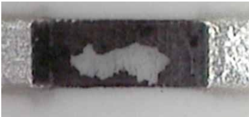
Figure 10. Photograph of catastrophically failed thick-film resistor due to the presence of hot spots caused by conducting material dispersion.
