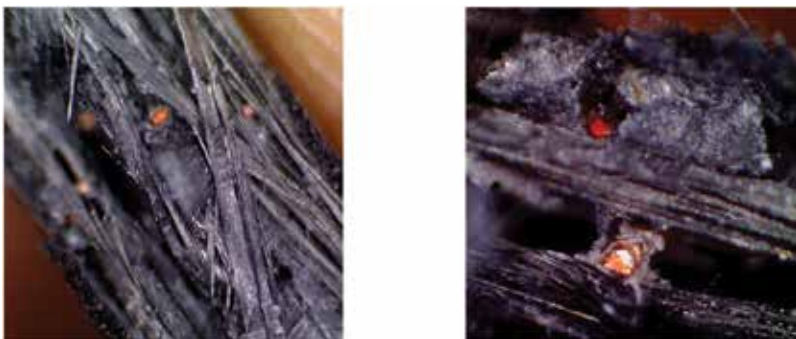
Figure 5. Tapering of conductive mesh (up to \times 200 magnification).
