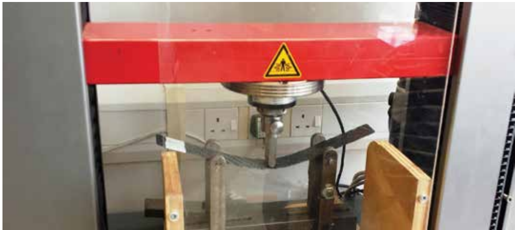
Figure 1. Flexural test equipment: universal testing machine.
