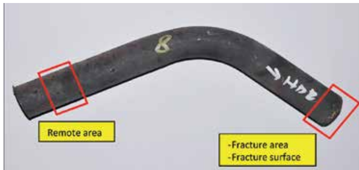
Figure 9. Dimensional reference of oxide thickness measurement.
