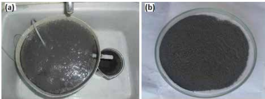
Figure 12. (a) Froth flotation separation with collector dose and (b) bottom fraction from froth flotation.
