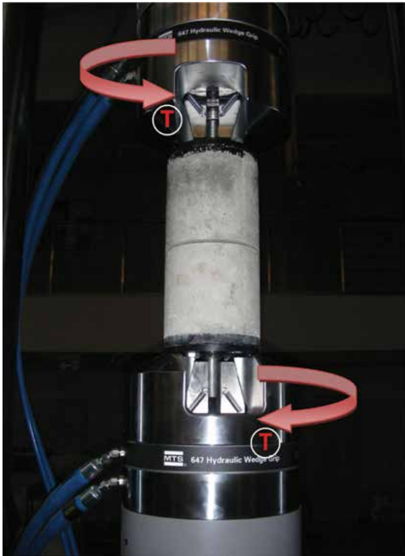
Figure 10. The experimental stand with the fixed specimen subjected to torsion; T, torque.
