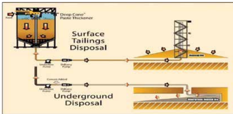
Figure 14. Paste thickening of treated neutralized effluent in the Coal mining AMD.
