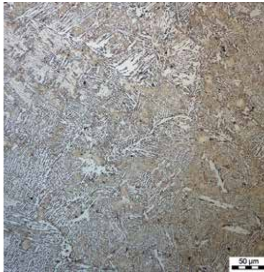
Figure 10. Microstructure of samples deformed in the solidification phase (core, “cold” grips).
