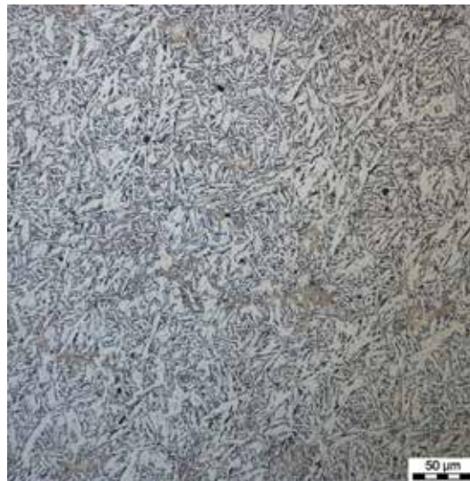
Figure 8. Microstructure of samples deformed in the solidification phase (core, “hot” grips).
