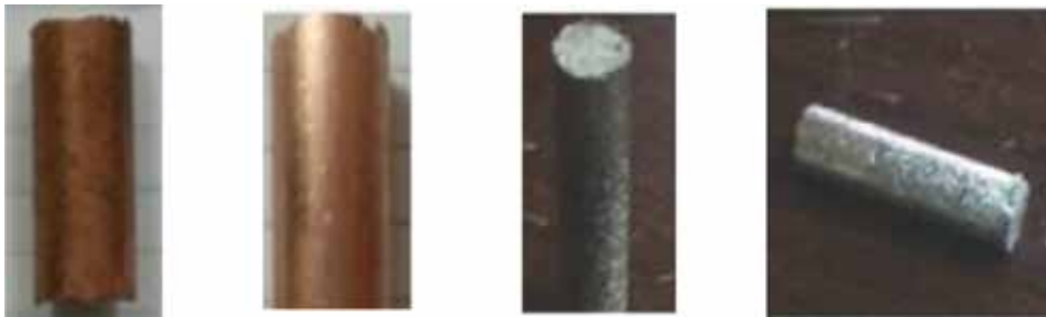
Figure 6. Samples of shafts produced from Al-Zn alloy and copper chips [19].
