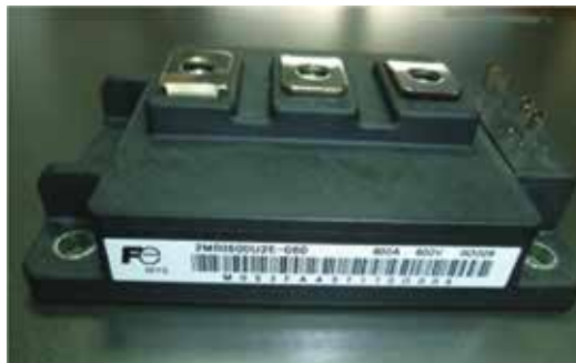
Figure 15. IGBT power transistors, T1/T2 type 2MBI 600 U2 E—060—FUJI [14].
