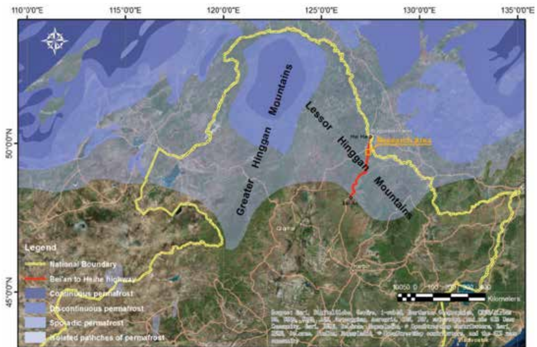
Figure 14. The permafrost distribution map at high latitudes in Northeast China and geographical location of the study area (data courtesy of the University of Zurich).
