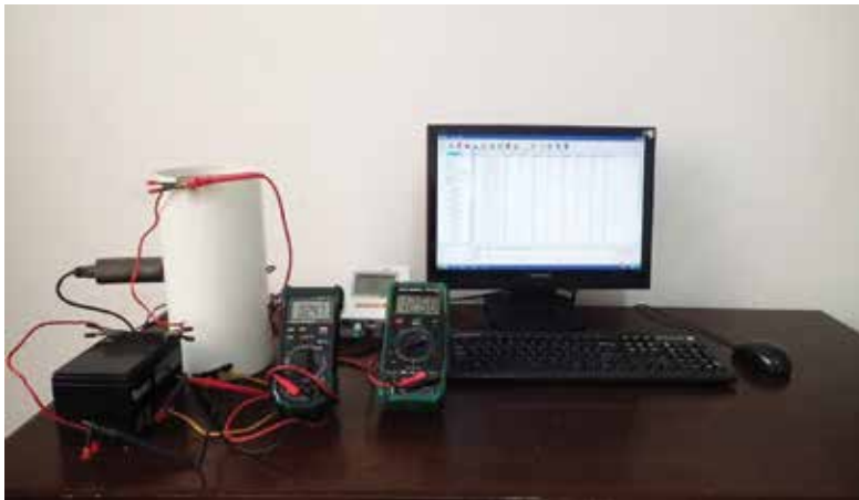
Figure 3. The LOGGER 3.0 system and the electrical resistivity measurement device.
