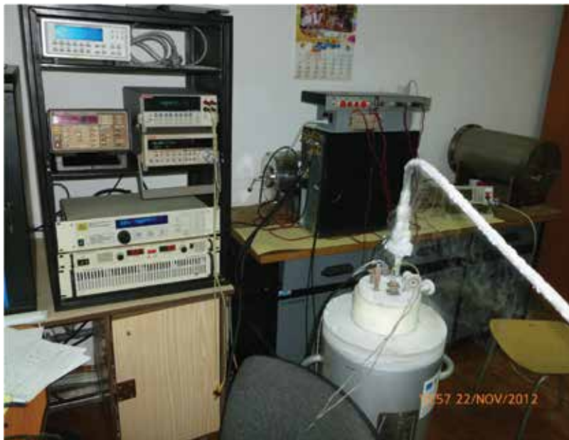
Figure 30. The experimental setup of the quench protection system of the superconducting coil during the experiments (the superconducting coil and the power supply are connected) [14].
