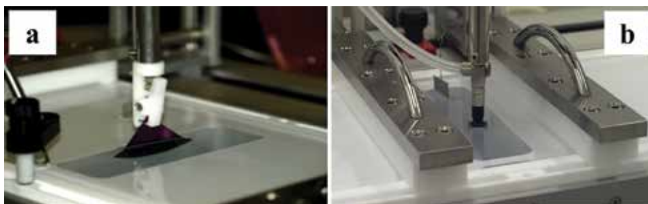
Figure 2. Langmuir-Blodgett (a) and Langmuir-Schaefer (b) transfer processes.
