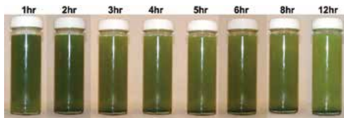
Figure 5. Nanoparticles sedimentation; CuO-reinforced nanofluids over time.
