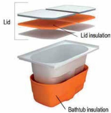
Structure of the insulated bathtub
