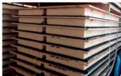
Well-insulated airtight wall panels backed with boards of rigid polyurethane foam
