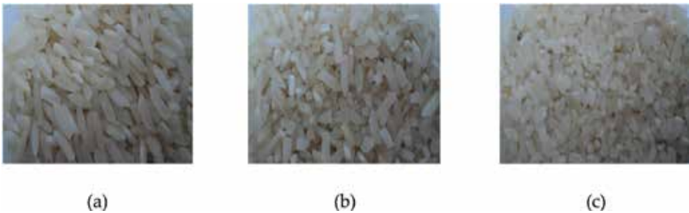
Figure 12. The rice grain with (a) 0%, (b) 50% and (c) 100% broken rate.
