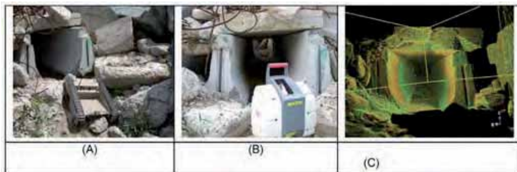
Fig. 17. A) Robot approaching a tunnel passage under rubble pile. B) Laser scanner captures high-resolution geometry data of all surfaces. C) Resulting "point cloud" of range data provides extremely accurate (ground-truth) model of actual rubble to support rubble classification and high-fidelity simulation environments for robot development and training.
