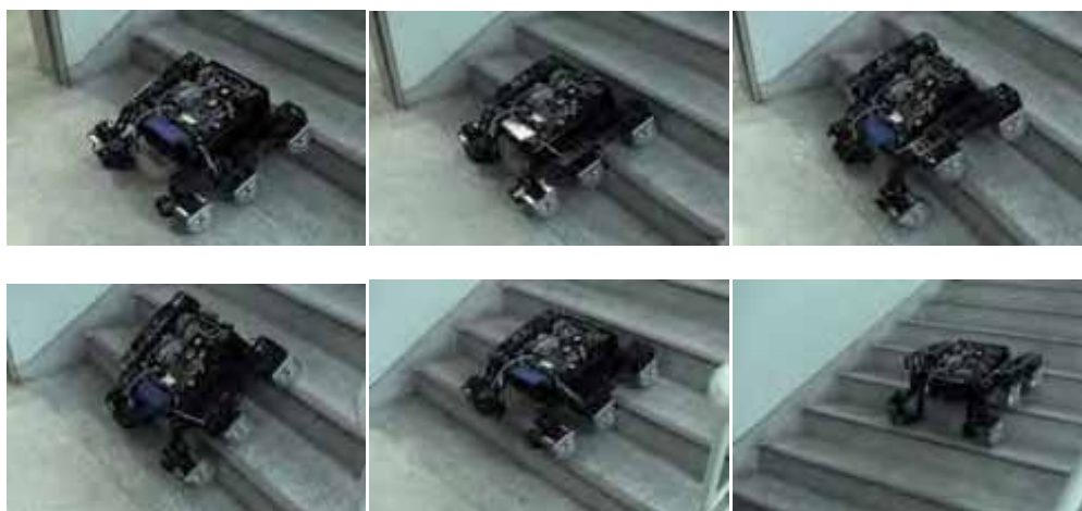
Fig. 21. Experiments for climbing the real stair
