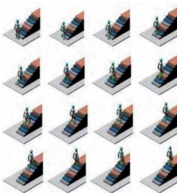
Fig. 19. Motion sequences of a humanoid robot climbing stairs
