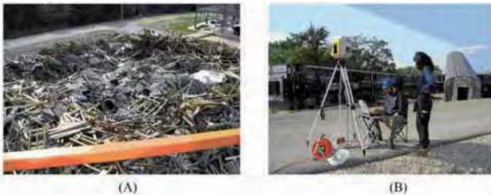
Fig. 14. (A).The wood pile was imaged using three ‘overhead’ scans and several ground-level scans. This view was taken from a scissors-lift. (B) Imaging the train wreck.
