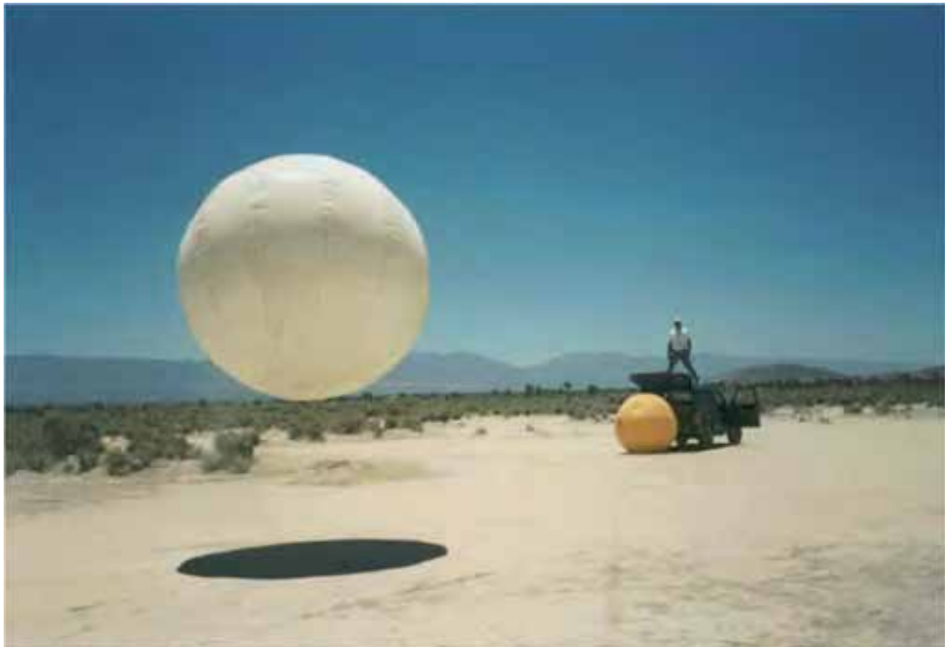
Fig. 15. Tumbleweed concept under testing (Antol et al., 2003)
