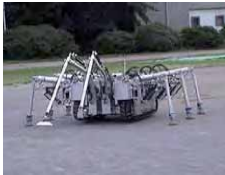
Fig. 1. COMET-III mine detecting six-legged robot
