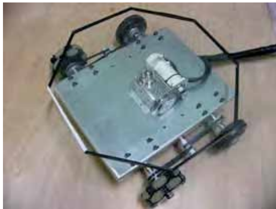
Fig. 9. Omnidirectional mobile platform with 4WD for experiments
