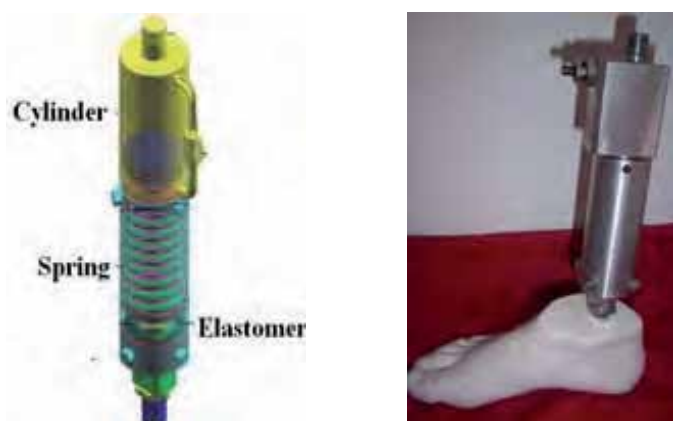
Fig. 15. Damper device for lower limb prosthetics
