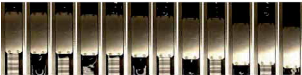
Fig. 26. Example of a passive locomotion by means of travelling waves in a magnetic fluid
