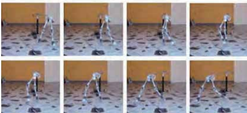
Fig. 12. Walking sequence for the robot UNROCA-II
