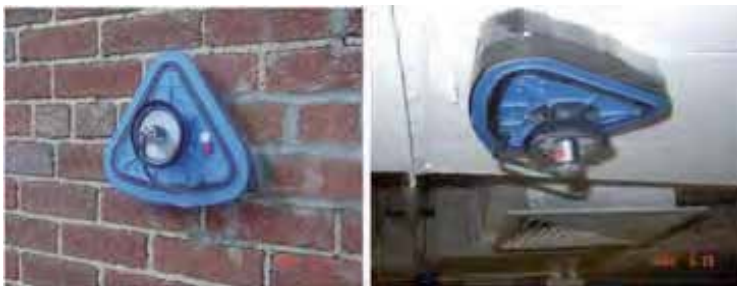
Fig. 16. The City-Climber prototype-II rests on a brick wall and sticks on a ceiling respectively
