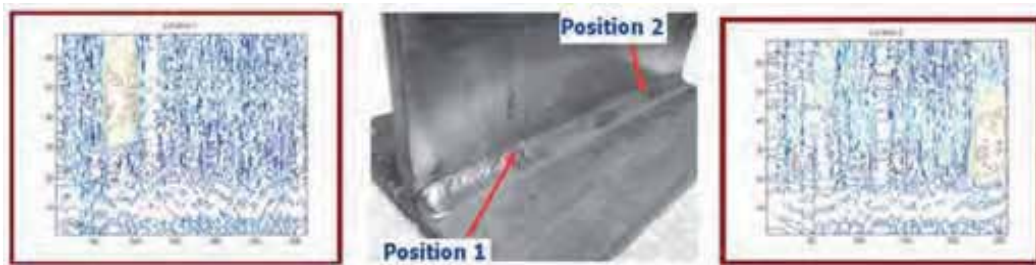
Fig. 17. A-scan results from ultrasonic creep. (Position1) defect at the beginning of the weld and (Position 2) defect at the end of the weld
