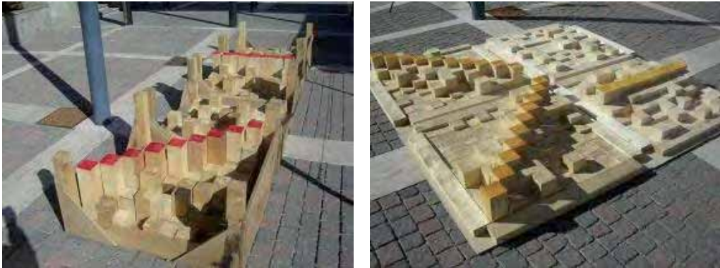
Fig. 2. Step Fields Provide Reproducible Terrain Challenges
