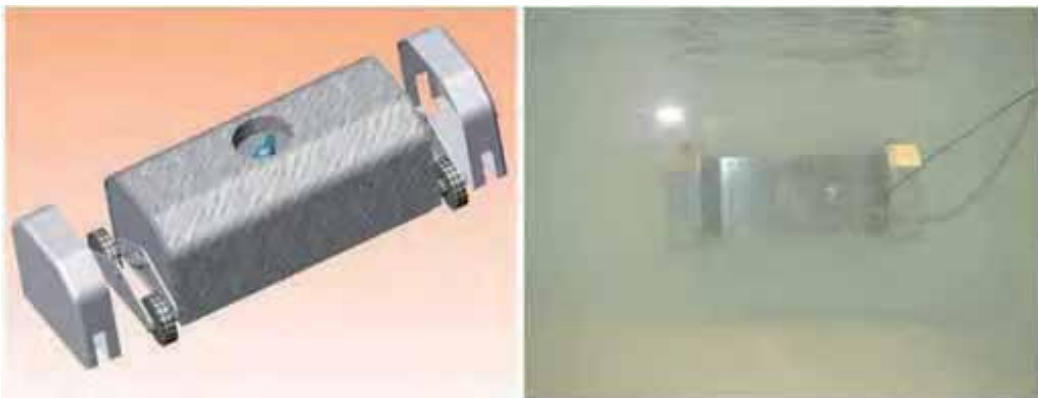
Fig. 2. Left: Solid drawing of RobTank; Right: Vehicle climbing on curved wall (3 metre diameter)
