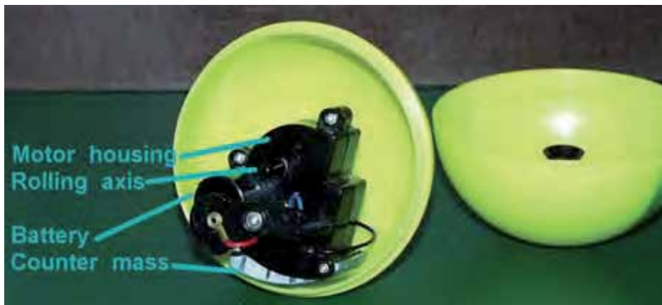
Fig. 8. 'Squiggleball' opened to show the interior parts (Image: TKK)
