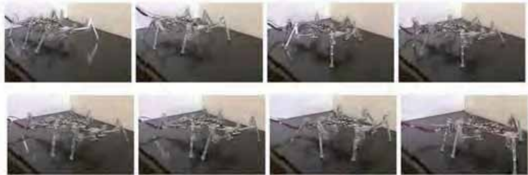
Fig. 17. Tripod gait walking of SMAR-III
