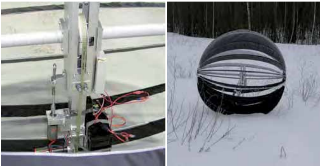
Fig. 18. (left) Thistle mechanism; (right), 1.3-m Thistle rolling on snow bed (TKK)
