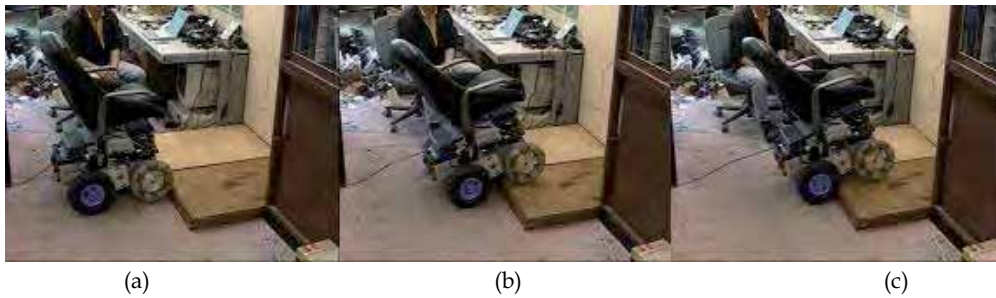
Fig. 18. Snapshots of the wheelchair in experiment: Climbing up a 90 mm step. Rear wheels failed to step up and all wheels slipped
