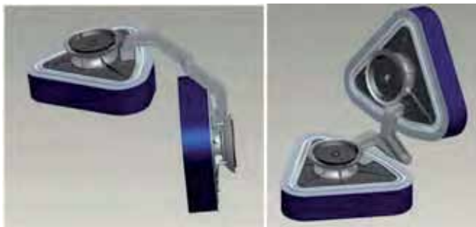
Fig. 15. Two robot modules connecting by a hinge in +90°, and -90° configurations, being able to make wall-to-wall, and wall-to-ceiling transitions
