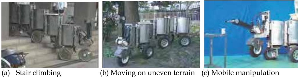
Fig. 1. Articulated body mobile robot “KR-II”, (first built in 1990, modified in 1997)
