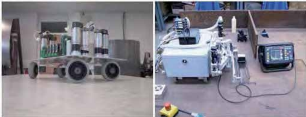
Fig. 15. Left: Platform to test robot motion and trajectory following capability. Right: Fully assembled robot performing NDT on a mock-up with Creep waves
