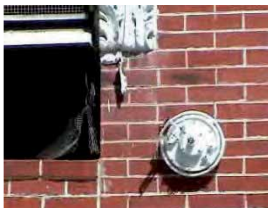
Fig. 13. City-Climber prototype-I approaching a window on brick wall, a CMU-camera is installed on a pan-tilt structure for inspection purpose.
