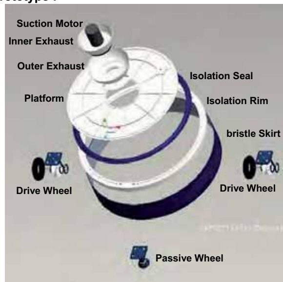
Fig. 12. Exploded view of City-Climber prototype-I.
