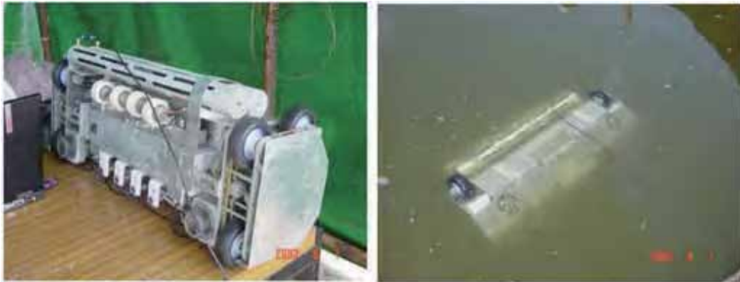
Fig. 5. Left: RobTank with full payload of 4 ultrasonic wheel probes, 4 compression probes and 2 rotating probes; Right: RobTank on the floor of a water storage tank, Sines oil refinery
