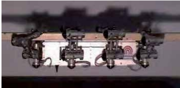
Fig. 20. SCORPION Robot using the PCR approach to climb along a beam
