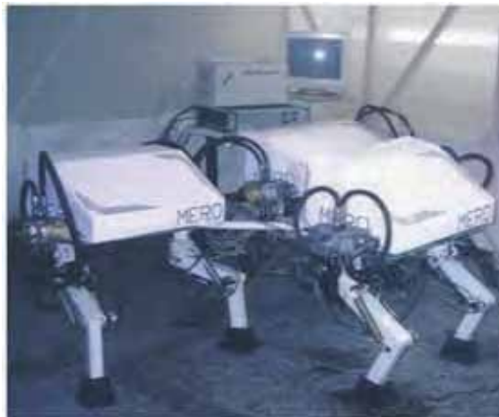
Fig. 5. MERO modular walking robot
