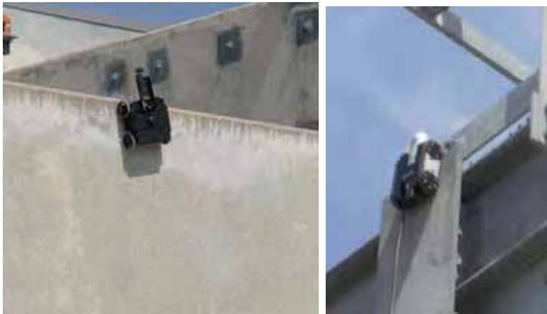
Fig. 5. Examples of wall-climbing robots
