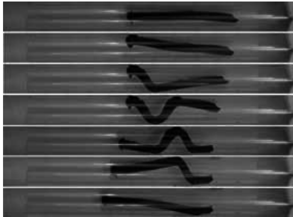
Fig. 17. Magnetizable elastic body (sample 1) in the travelling magnetic field
