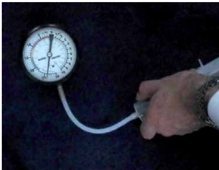
Fig. 3. A 60cc syringe can generate close to one atmosphere (30 in = 760 mm Hg) of negative pressure, dispelling the myth that syringe suction is “safer” than machine suction.
