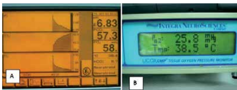
Fig. 11. A: Neurotrend and B: Licox system. Neurotrend is capable of measuring brain temperature, brain pH, PtiO 2 , PtiCO 2 and HCO 3 whereas Licox only measures PtiO 2 and brain temperature.
