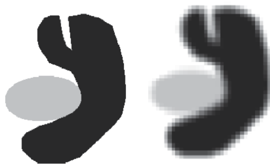
Fig. 6. Illustration of partial volume effect. (Left) Ideal image; (Right) Acquired image (Images provided courtesy of D.L. Pham).
