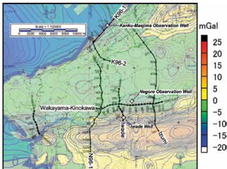
Figure 19. Overlaid images of geography and gravity anomaly trend [27] around the southern flank of the Izumi Mountains.
