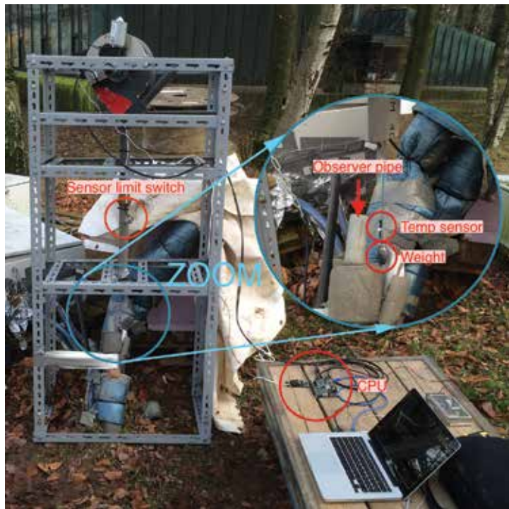
Figure 30. The implemented system before the beginning of the acquisition process in a BHE.
