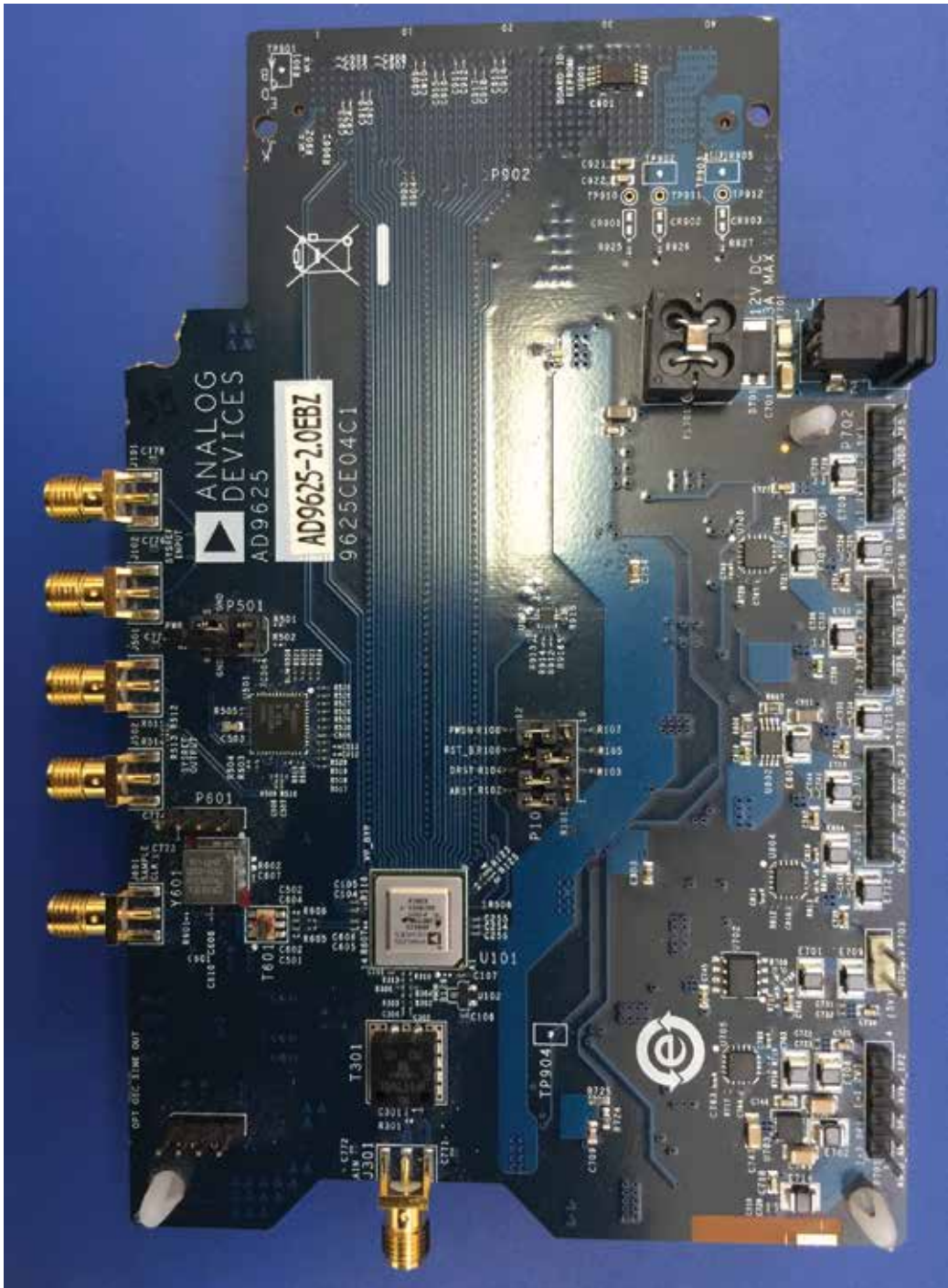
Figure 3. AD9625-2.0EBZ Evaluation Board.
