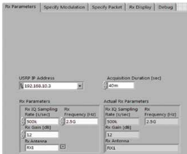
Figure 8. Front panel of USRP receiver/Rx parameter.
