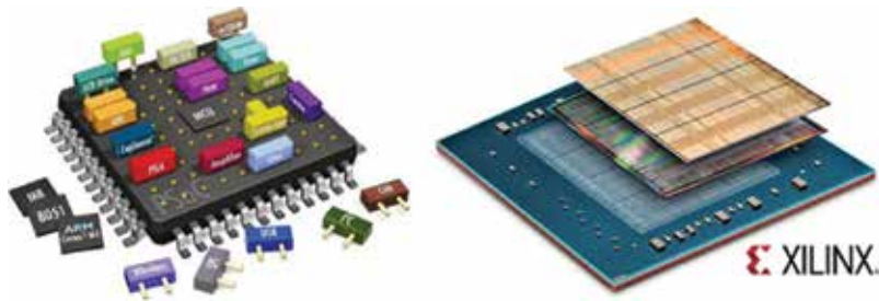
Figure 11. Examples of SoCs (picture courtesy of Cypress and Xilinx).
