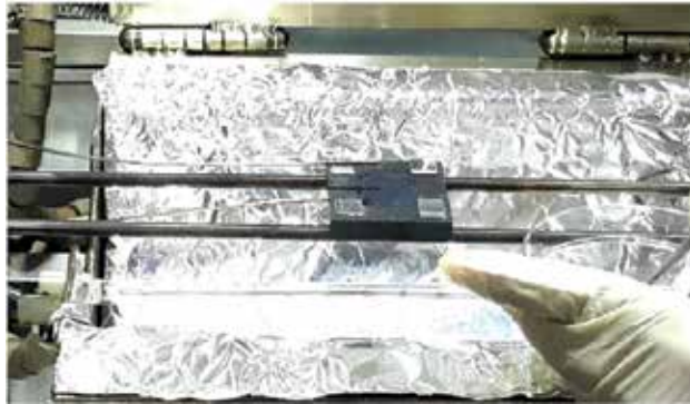
Figure 4. Inside view of the CSS chamber with spacers placed on top of bottom holder.
