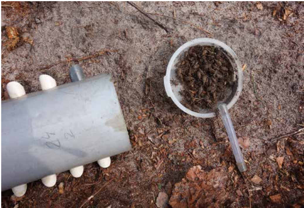
Photo 5. Hyllobius abietis beetles collected by IBL-4 trap, visible dispenser in the form of tube filled with synthetic attractant.
