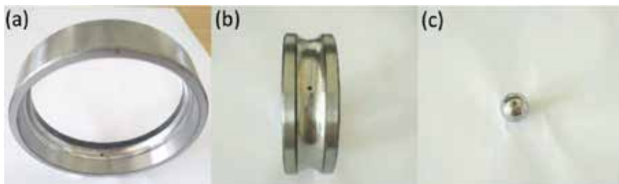
Figure 19. Simulated bearing faults: (a) outer race fault; (b) inner race fault; and (c) ball fault.
