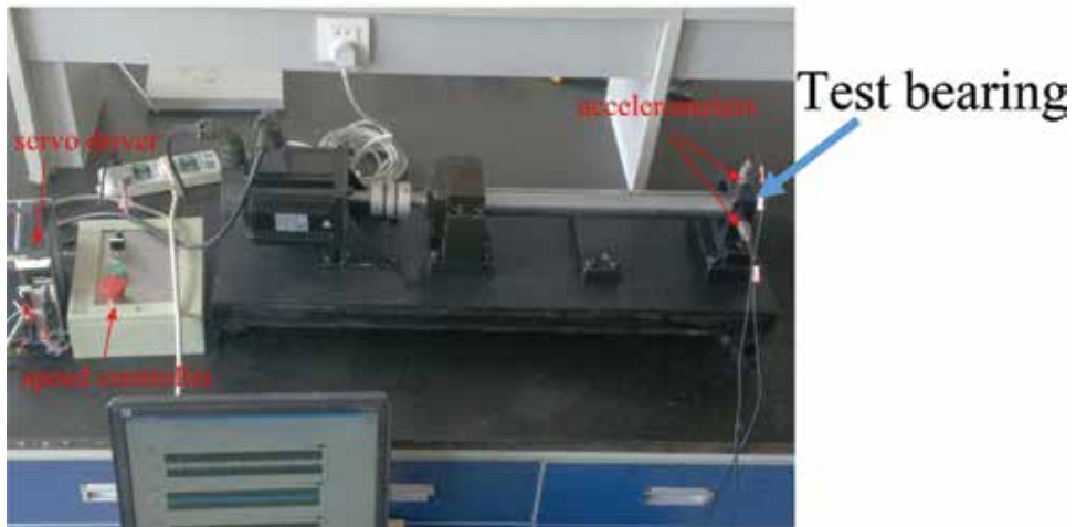
Figure 18. A graphical illustration of the bearing fault simulation test rig.
