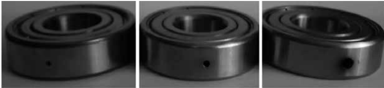
Figure 2. Damaged bearings used in the experimental tests. From left to right holes of 1.0 mm, 2.0 mm, and 3.0 mm.
