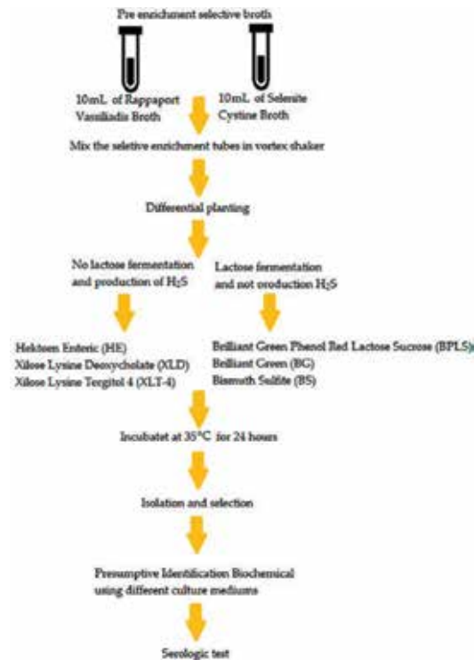
Figure 7. Procedure for differential plating and biochemical identification.
