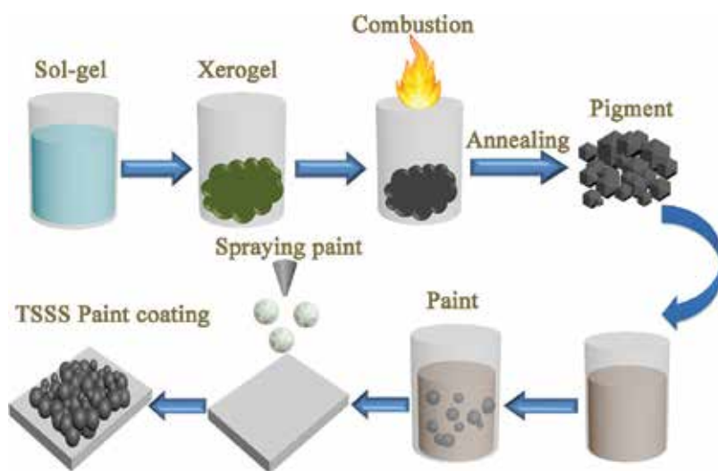
Figure 1. Spectrally selective paint coatings based on spinel ceramic pigments are fabricated [14].
