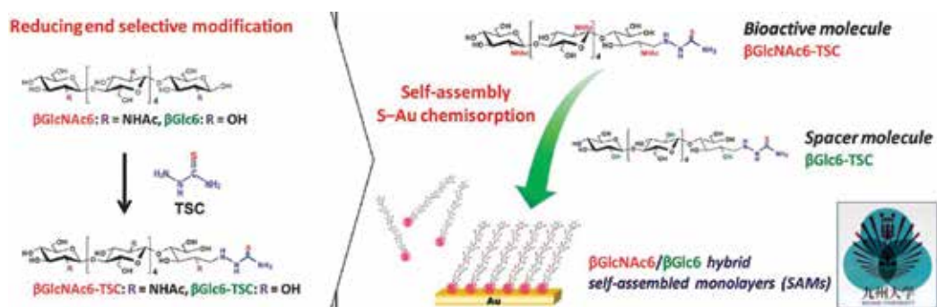
Figure 6. Schematic illustration of thiosemicarbazide (TSC)-derivatization and self-assembly immobilization of GlcNAc6 and GlcN6. The photograph is an optical image of carbohydrate-SAMs. Reprinted with permission from Ref. [53], Copyright 2011, The Royal Society of Chemistry.
