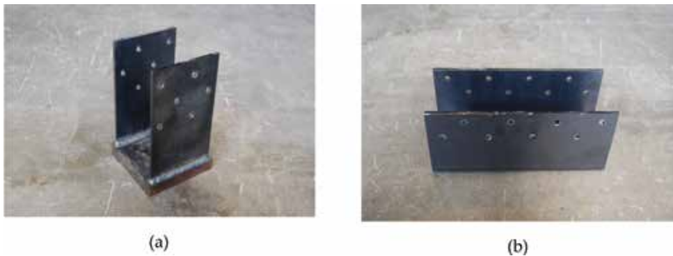
Figure 3. Connections: (a) tensile-type and (b) shear type.
