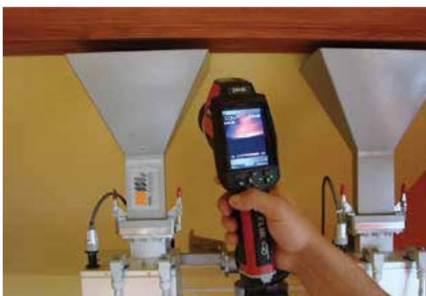
Figure 9. Monitoring the temperature of the wood by thermal imaging can cause distortions to the view of the situation: the areas of high temperature, visible on the screen, can cover layers of much lower temperature, harmless to the larvae (photo by CARSEKT).
