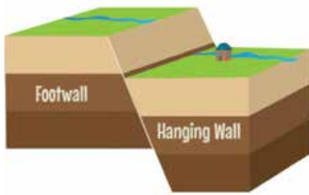
Figure 5. Normal fault graphical presentation and mechanism [7].
