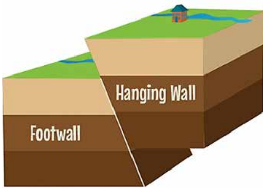
Figure 6. Reverse fault graphical presentation and mechanism [7].
