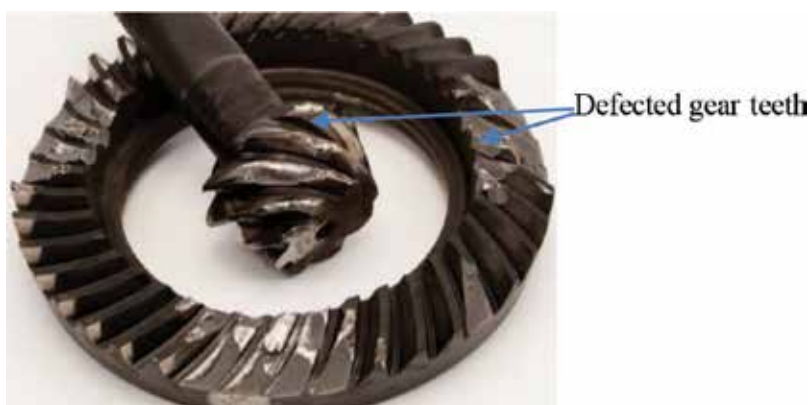
Figure 8. Example of the gear defects [30].
