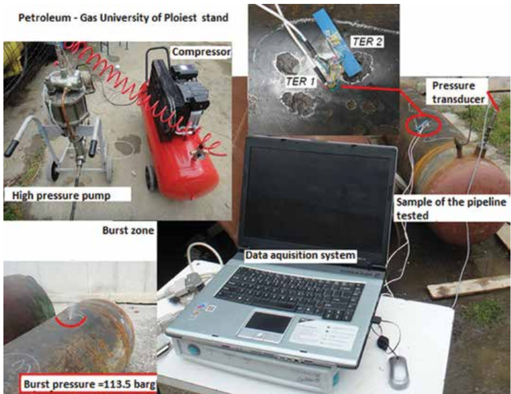
Figure 8. Main components of the stand used to inner pressure test of pipe samples.
