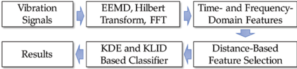
Figure 2. The procedures of the proposed fault diagnosis approach for rotating machinery.
