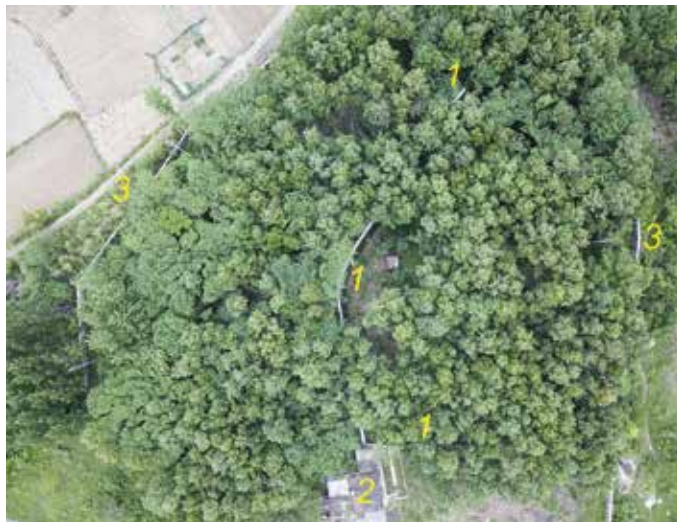
Figure 3. The bird’s eye view of the forested Nandadish watershed taken at May 2018. 1-trench with layered troughs; 2-block divider; 3-house for discharge measuring structures.
