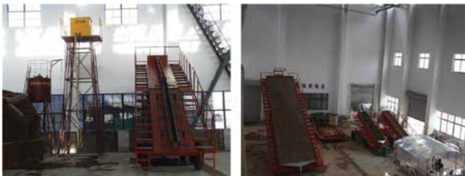
Figure 6. Experimental variant slope soil tank in Institute of Soil and Water Conservation Chinese Academy of Sciences.
