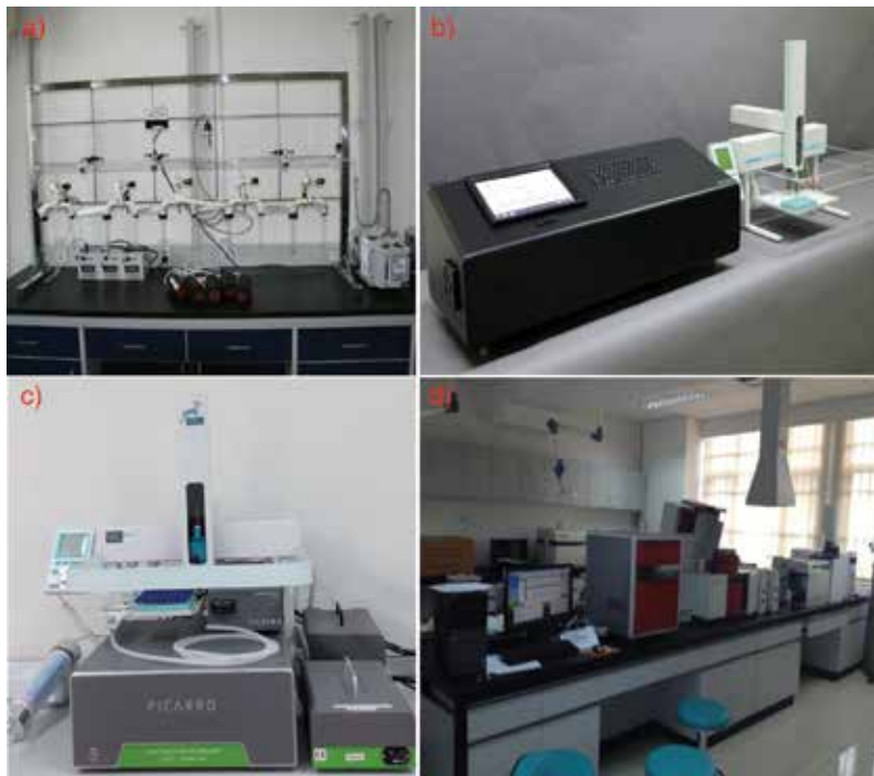
Figure 26. Instruments adopted in isotope analysis of water samples: (a) a vacuum extraction system (LI-2000, LICA, China); (b) a liquid water isotope analyzer (908-0008, LGR, USA); (c) a liquid-gas water isotope analyzer (L2120-i, Picarro, USA); (d) IsoPrime100.
