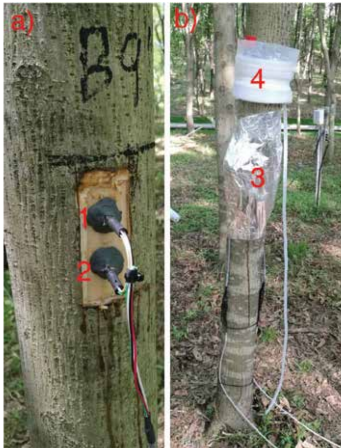
Figure 7. Installation of thermal dissipation probes: (a) a set of TDP includes a heated needle (1) and a reference needle (2); (b) the reflective bubble shield (3) was wrapped around the TDP probe to avoid monitoring errors caused by direct sunlight and rainfall leaching, and a collection collar (4) for stem flow was installed above the TDP to stop stem flow entering.
