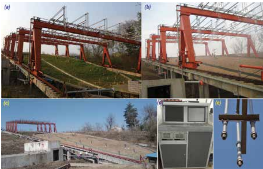
Figure 19. Rainfall simulator system in Hydrohill: (a) before the rainfall simulating; (b) during the rain simulating; (c) after the rainfall simulating event (1-an impounding reservoir supplying the rainfall simulator system, 2-a water supplying pipe); (d) the rainfall simulator control platform located in the gauging room; (e) combination of different sizes of sprinkle nozzles.
