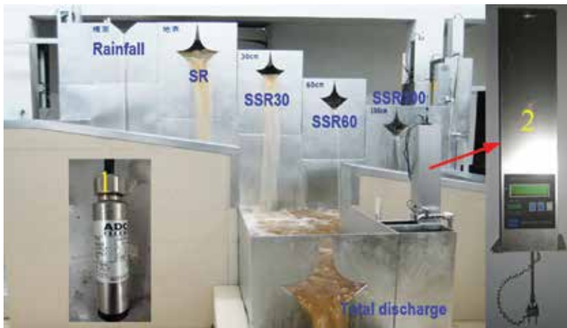
Figure 15. The discharge measuring structures of renovation version and the instrumentation for its water heads. 1-probe-type water level gauge; 2-tracking gauge for the real-time water head process.
