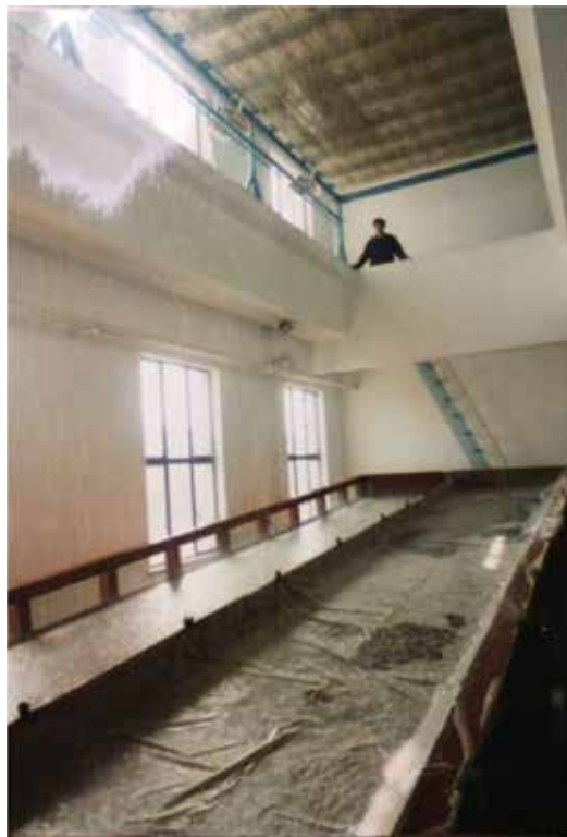
Figure 3. The experimental variant slope soil tank in the runoff laboratory of Institute of Geography.
