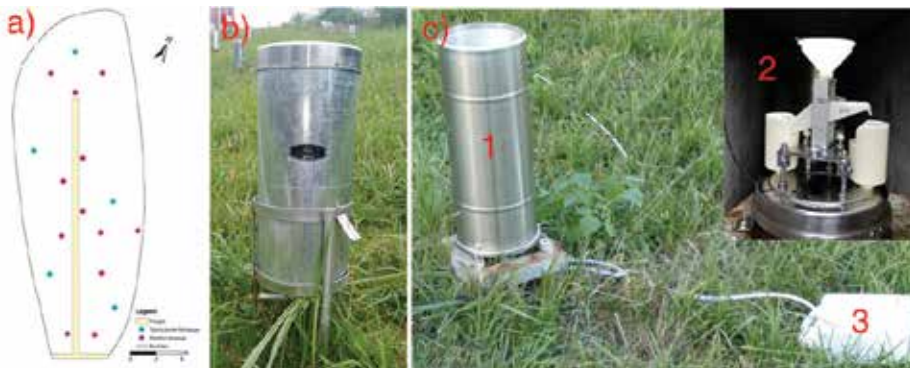
Figure 14. Instrumentation for precipitation measurement in Hydrohill: (a) locations of 12 standard rain gauges and 5 tipping bucket rain gauges; (b) a standard rain gauge; (c) a tipping-bucket rain gauge. 1-external structure, 2-internal structure, 3-a plastic pot used to collect total precipitation of each event.
