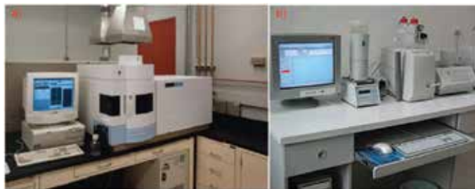
Figure 25. Instruments adopted in hydrochemistry analysis of water samples: (a) inductively coupled plasma optical emission spectrometry (ICP-OEC); (b) ion chromatography (ICS-2100, DIONEX, USA).
