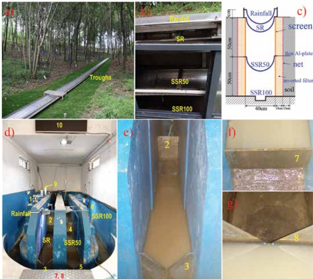
Figure 5. Instrumentation for runoff measurement in Nandadish: (a) Main trench with troughs (not shown), (b) the branch trench with four troughs (previously Figure 13c ), (c) schematic figure illustrating various troughs, (d) discharge measurement structures for different runoff components from troughs 1 for rainfall; 2 and 3 for surface runoff; 4 and 5 for interflow (50 cm below the soil surface); 6 for interflow and groundwater flow (down to bedrock); 7 and 8 for total runoff (weirs are shown (f) and (g)). 1, 3, 5, 6, and 8 are 90° V-notch weir; 2, 4 and 7 are the full width rectangular weirs; 9 is the probe-type water level gauge; 10 is a video for monitoring the runoff processed, (e) combination of a 90° V-notch weir and a full width rectangular weir for SR, SSR50, and the total runoff, (f) the full width rectangular weir for total runoff, (g) the 90° V-notch weir for total runoff.
