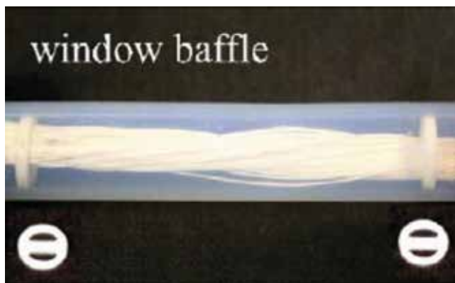
Figure 9. Hollow fiber module with window baffles [38].
