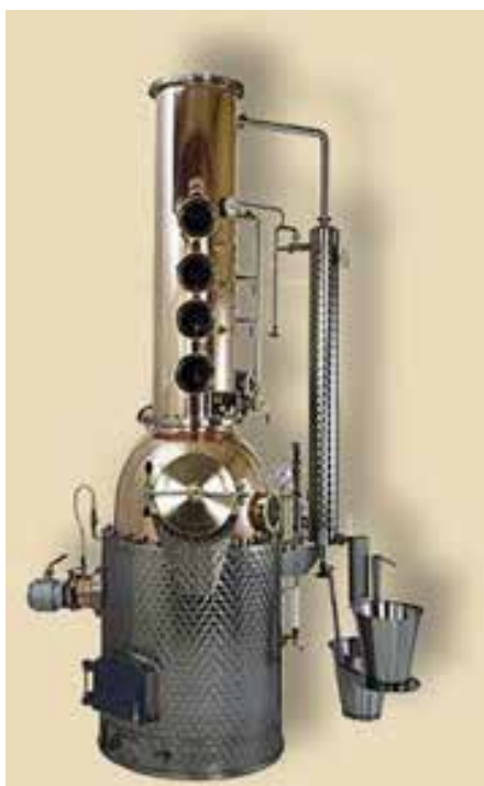
Figure 4. Steam-fired batch distillation column still with three trays and dephlegmator above them. Reflux rate is varied by changing the cooling rate in dephlegmator.
