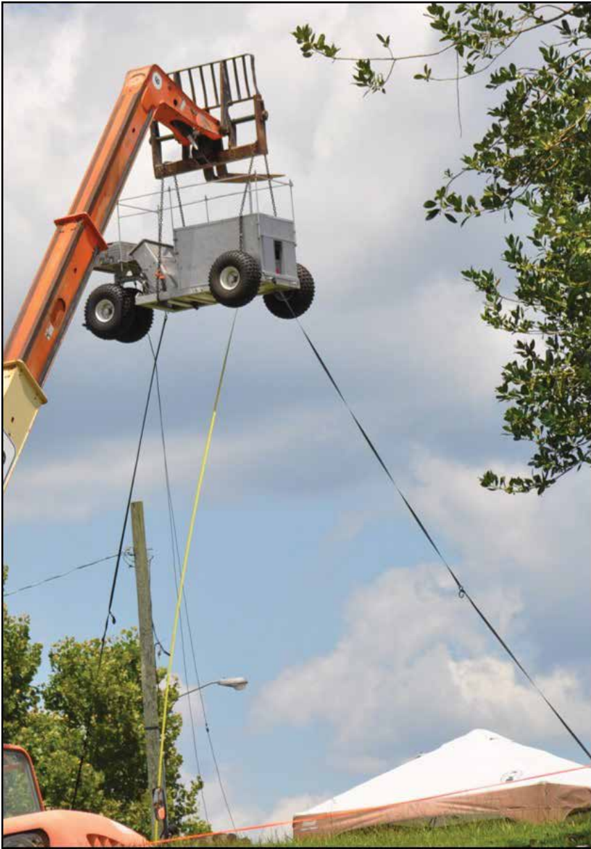
Figure 7. The PFTNA system background measurements (up to 6.7 m above the ground) [79].
