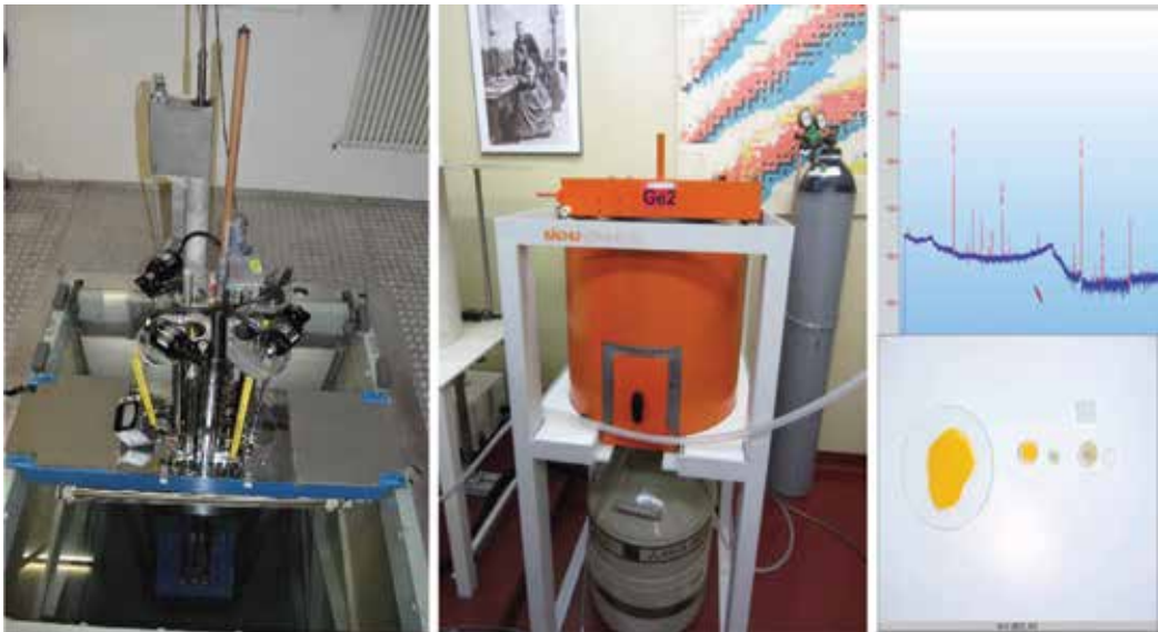
Figure 1. Equipment for NAA. Swimming pool reactor (left) gamma-ray spectrometer with lead shielding (middle) gamma-ray spectrum (above right) curry sample and sample device for the irradiation [4].
