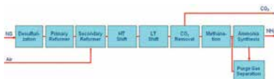
Figure 6. Block diagram of ammonia plant.
